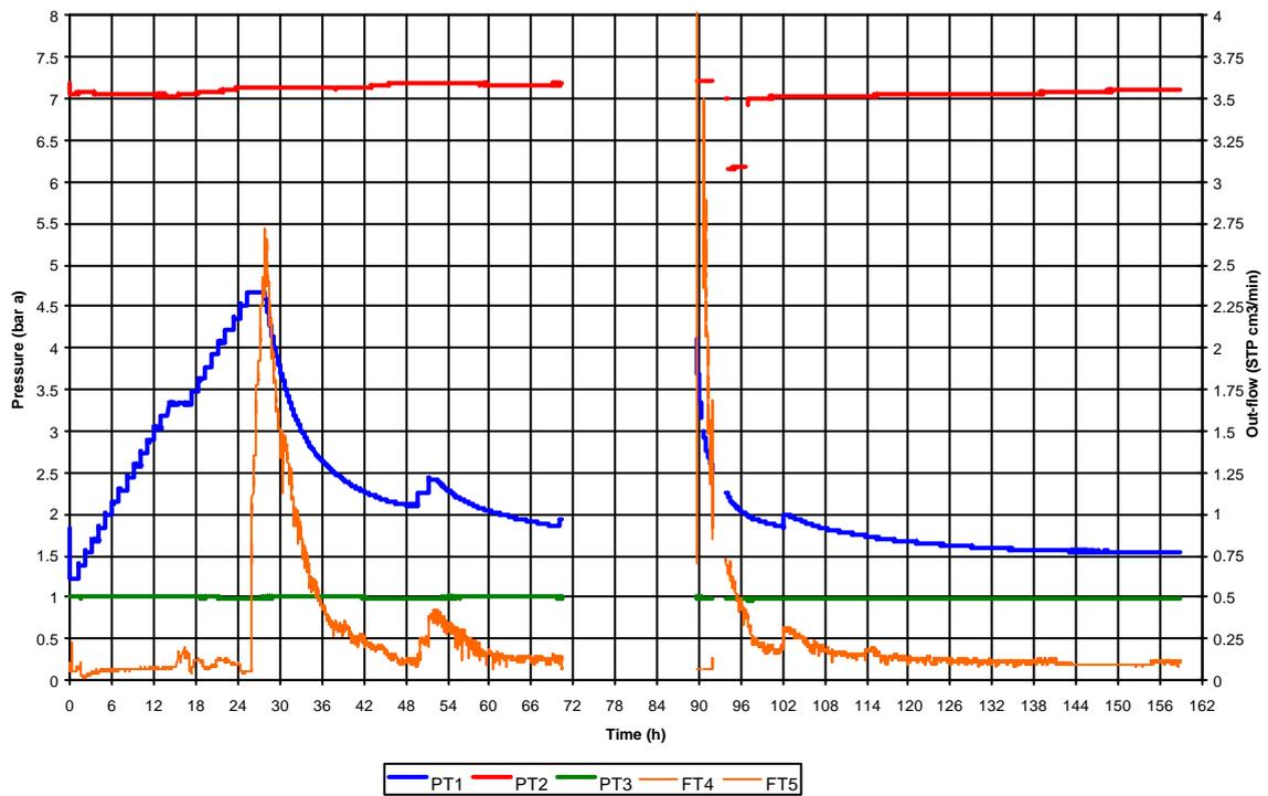
Figure 6: Pressure / Out-flow versus time for saturated sample within elastic membrane
