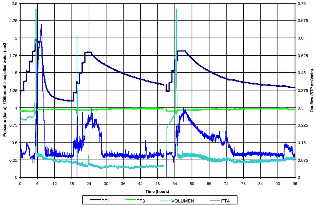
Figure 7: Pressure / Out-flow versus time for saturated sample within rigid jacket
