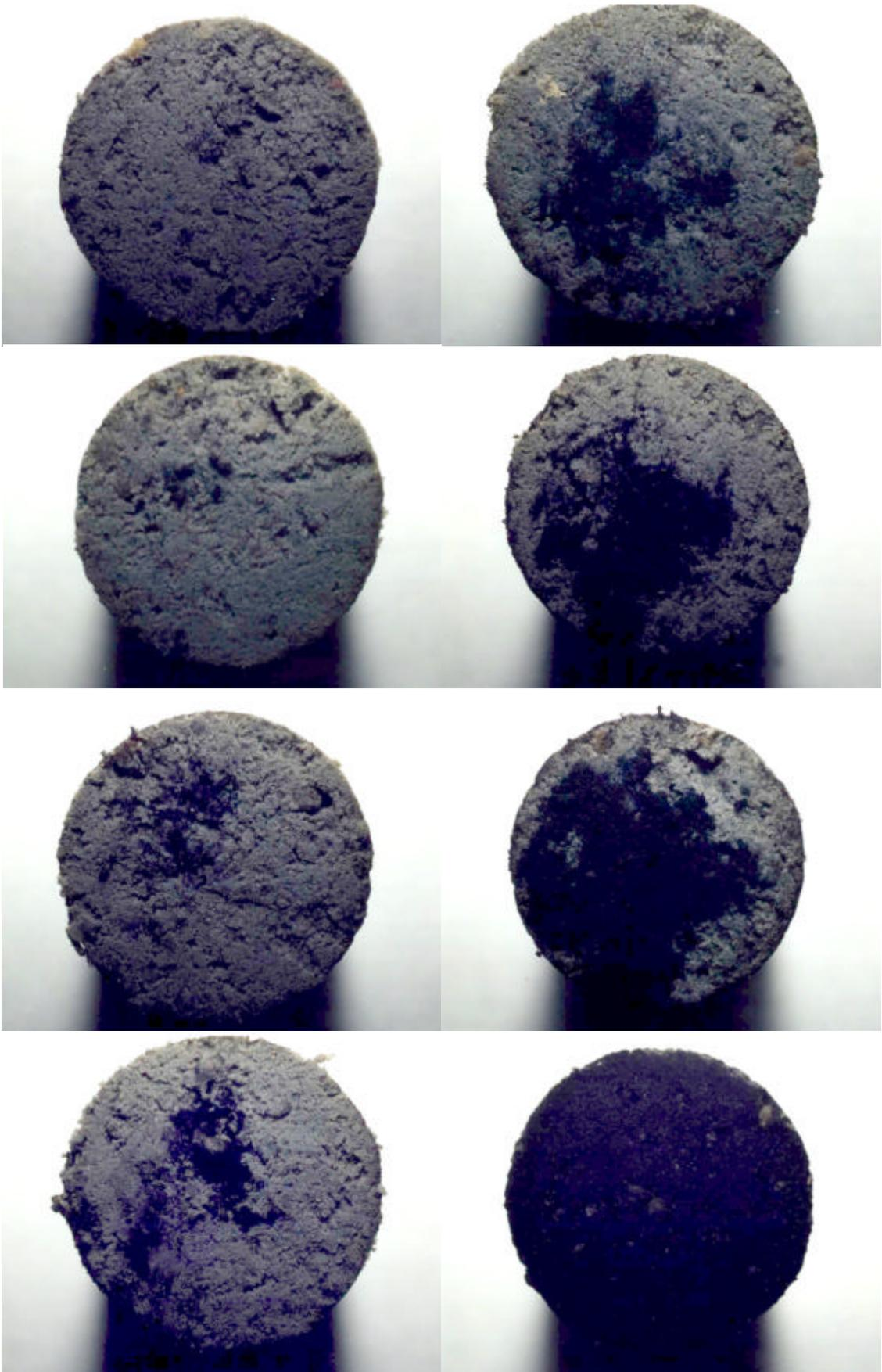
Figure 9: Sample exposed to  $\text{SH}_2$  flow: Details of the sections.
