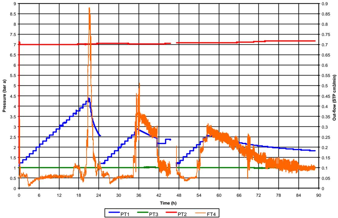
Figure 5: Pressure / Out-flow versus time for 0.9 saturation sample
