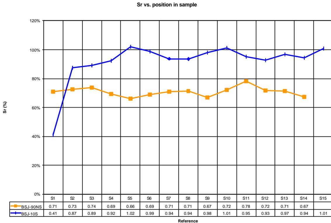
Figure 4: Measured saturation vs. position in sample (S1: inlet).
