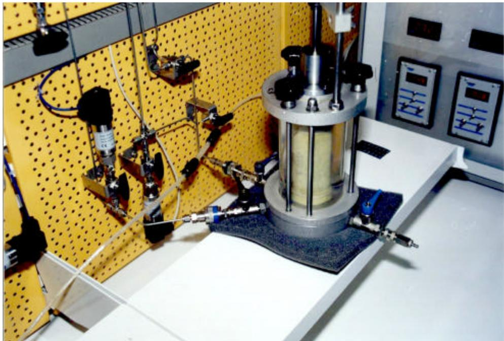
Figure 12: Installation of the sample: detail of the connection to the measuring system.
