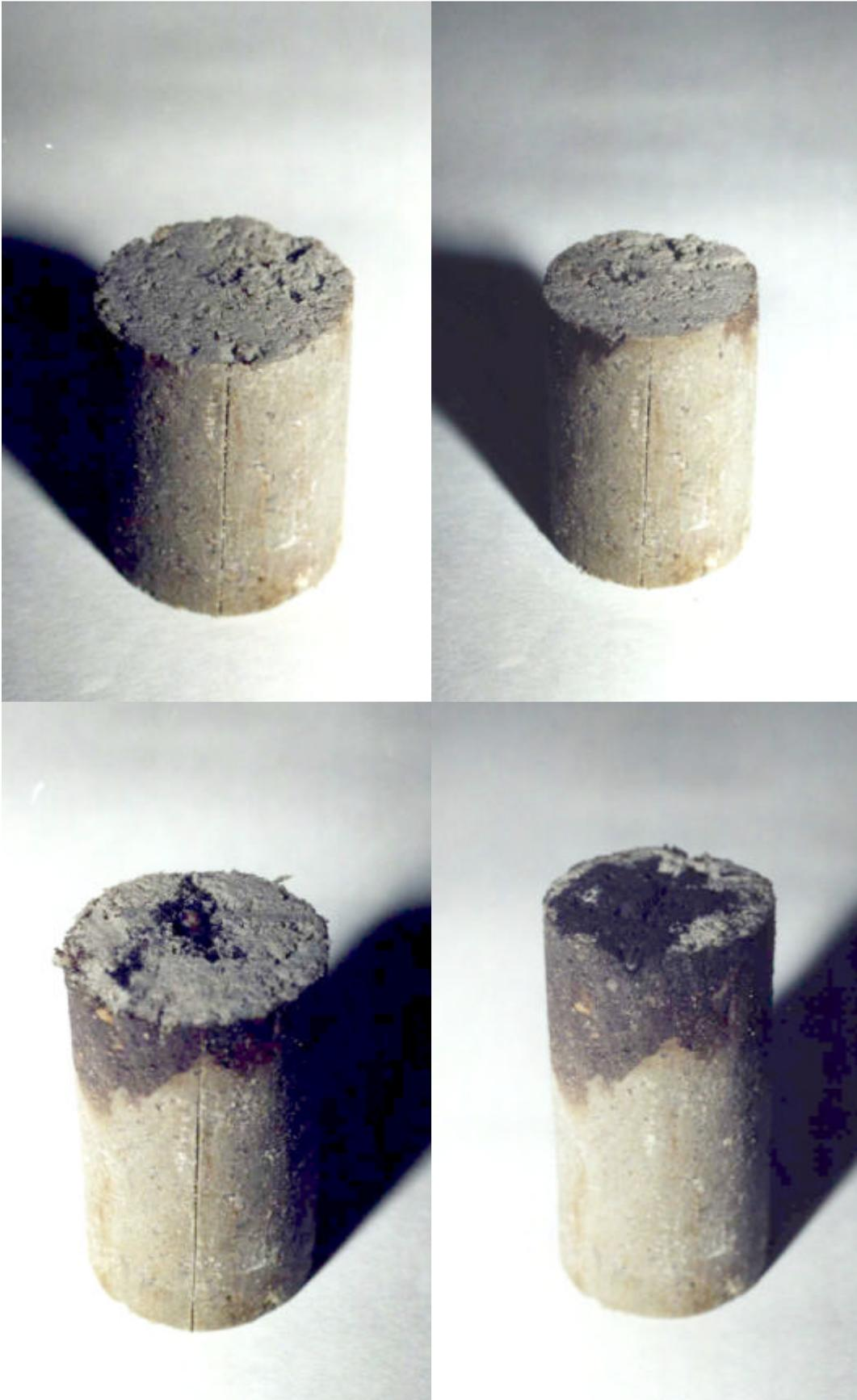
Figure 10: Sample exposed to SH<sub>2</sub> flow: Details of the cutting sequence.
