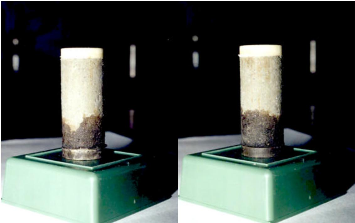
Figure 8: Sample exposed to SH<sub>2</sub> flow: views at 180° before cutting.
