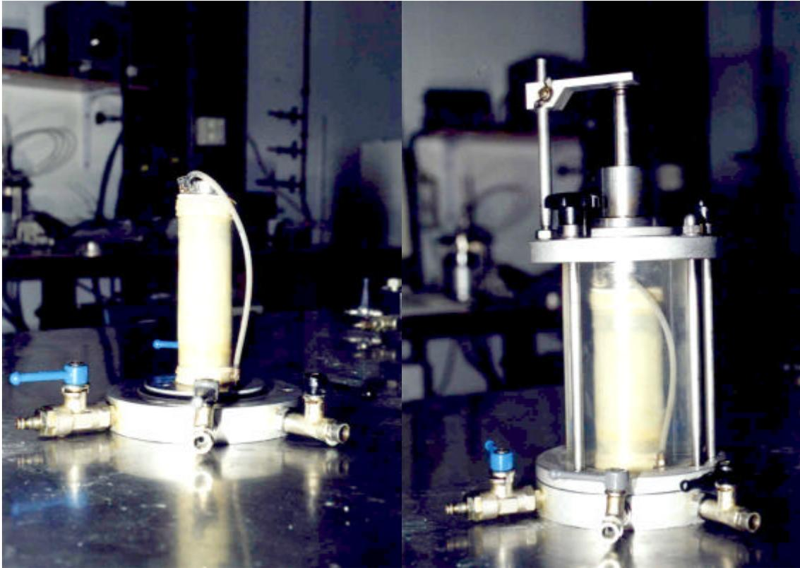
Figure 2: Installation of the sample in the triaxial cell.
