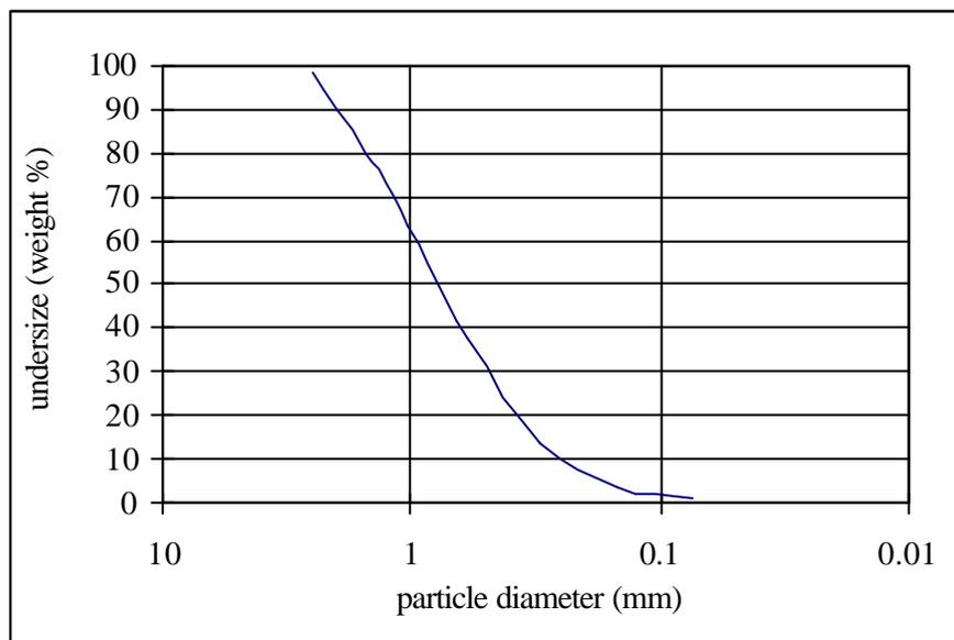
Figure 1: Particle size distribution of the quartz sand
