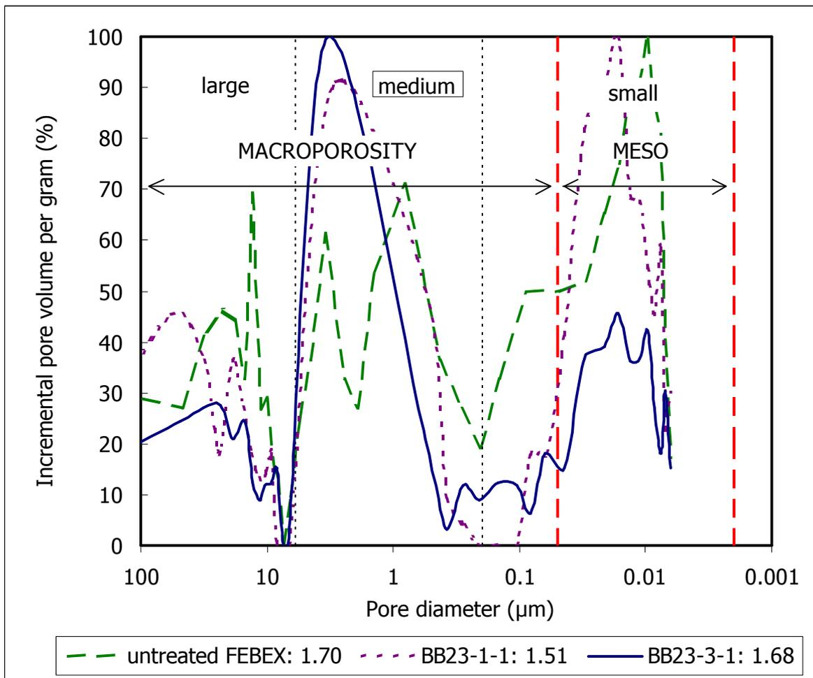
**Figure 24: Incremental porosimetric curve for untreated FEBEX bentonite and two samples from Grimsel, with indication of dry density in  $\text{g/cm}^3$**
