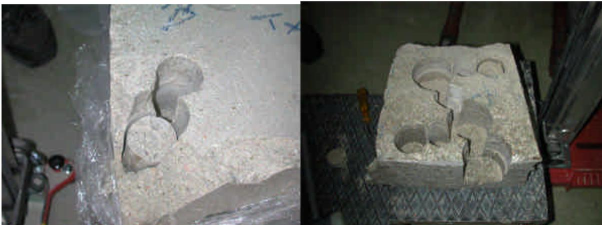
**Figure 8: Drilling of blocks to obtain samples for the THM determinations**
