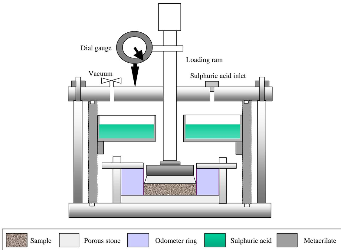
**Figure 34: Schematic cross section of an oedometric cell with deposit for solutions**
