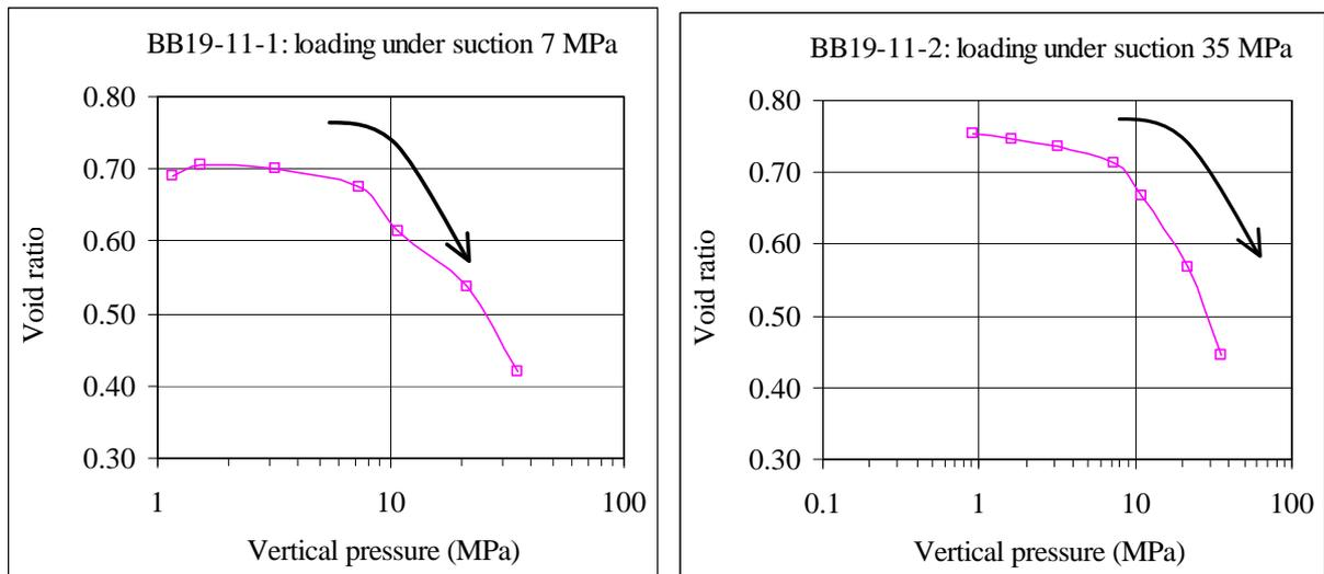
**Figure 43: Oedometric curves of the tests performed in samples from block BB19-11**
