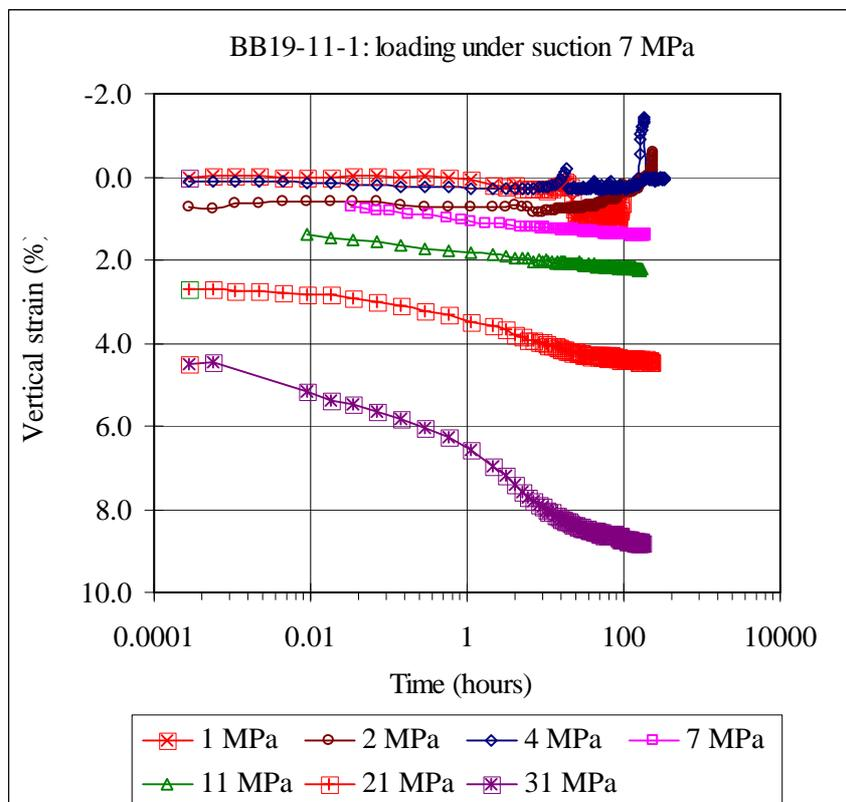
**Figure 38: Evolution of strain during the different steps of the process of loading under suction 7 MPa for sample BB19-11A-1**
