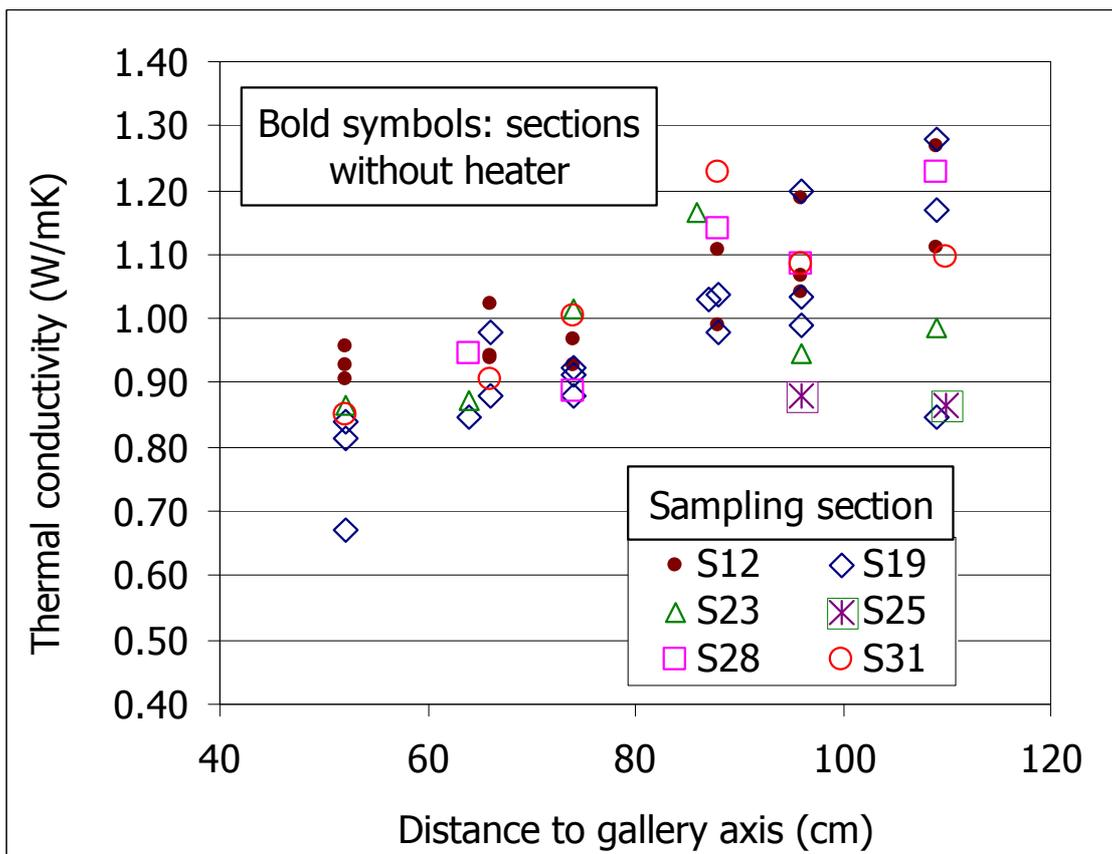
Figure 46: Thermal conductivity along radius of different sections
