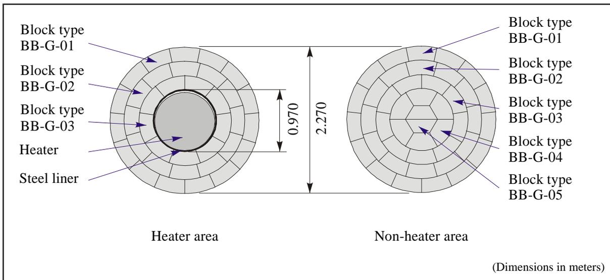
**Figure 2: Geometry of the clay barrier in the FEBEX *in situ* test at GTS (ENRESA 2000)**
