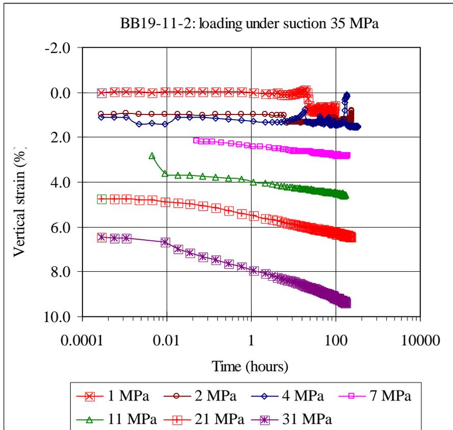
**Figure 39: Evolution of strain during the different steps of the process of loading under suction 35 MPa for sample BB19-11A-2**
