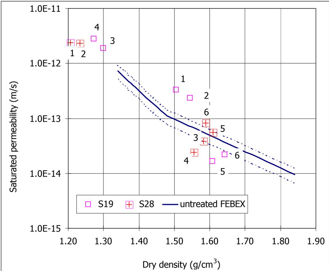
**Figure 28: Hydraulic conductivity as a function of dry density for samples of sections S19 and S28. The lines correspond to the empirical fittings obtained with equations [3] and [4] (the position of the samples is indicated with correlative numbers from 1 –closest to gallery wall– to 6 –closest to heater–)**
