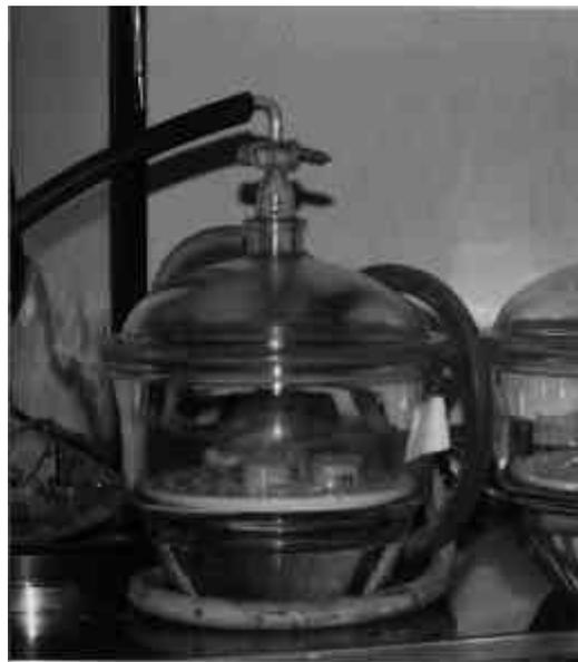
**Figure 14: Desiccator with the trimmed samples inside**
