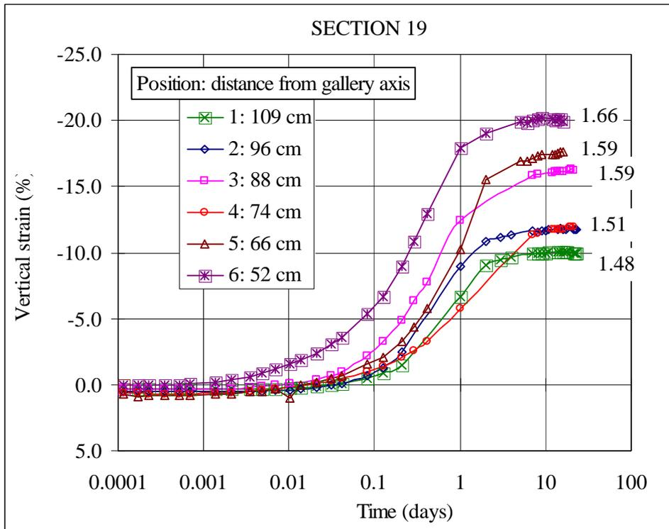
**Figure 31: Evolution of vertical strain during saturation under vertical load 0.5 MPa for samples from section S19 (the initial dry density of the samples is indicated in  $\text{g/cm}^3$ )**
