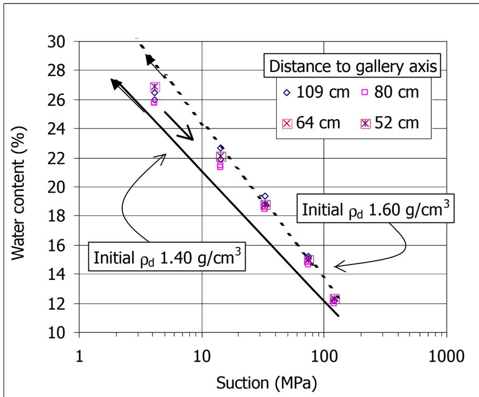
Figure 19: Evolution of water content in a drying path for samples from section S23. The lines correspond to untreated FEBEX bentonite in wetting paths (obtained with equation [1])
