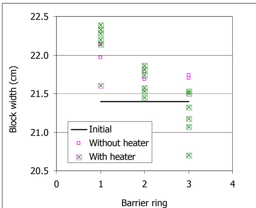
**Figure 4: Radial dimension of the blocks measured *in situ* during dismantling in three different rings (1: external; 2: intermediate; 3: inner)**
