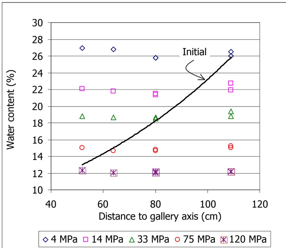
Figure 15: Water contents reached under different suctions for samples from section S23
