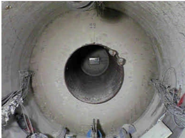
**Figure 3: Aspect of the bentonite barrier after extraction of the heater**
