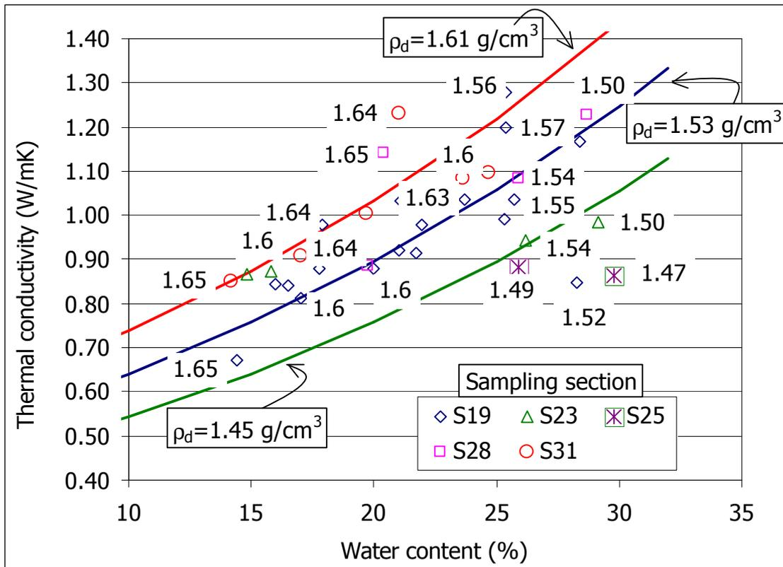
Figure 47: Thermal conductivity values measured in blocks from Grimsel (dry density indicated in  $\text{g/cm}^3$ ) and theoretical fittings obtained with Equation 6
