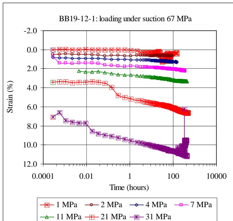
**Figure 40: Evolution of strain during the different steps of the process of loading under suction 67 MPa for sample BB19-12A-1**
