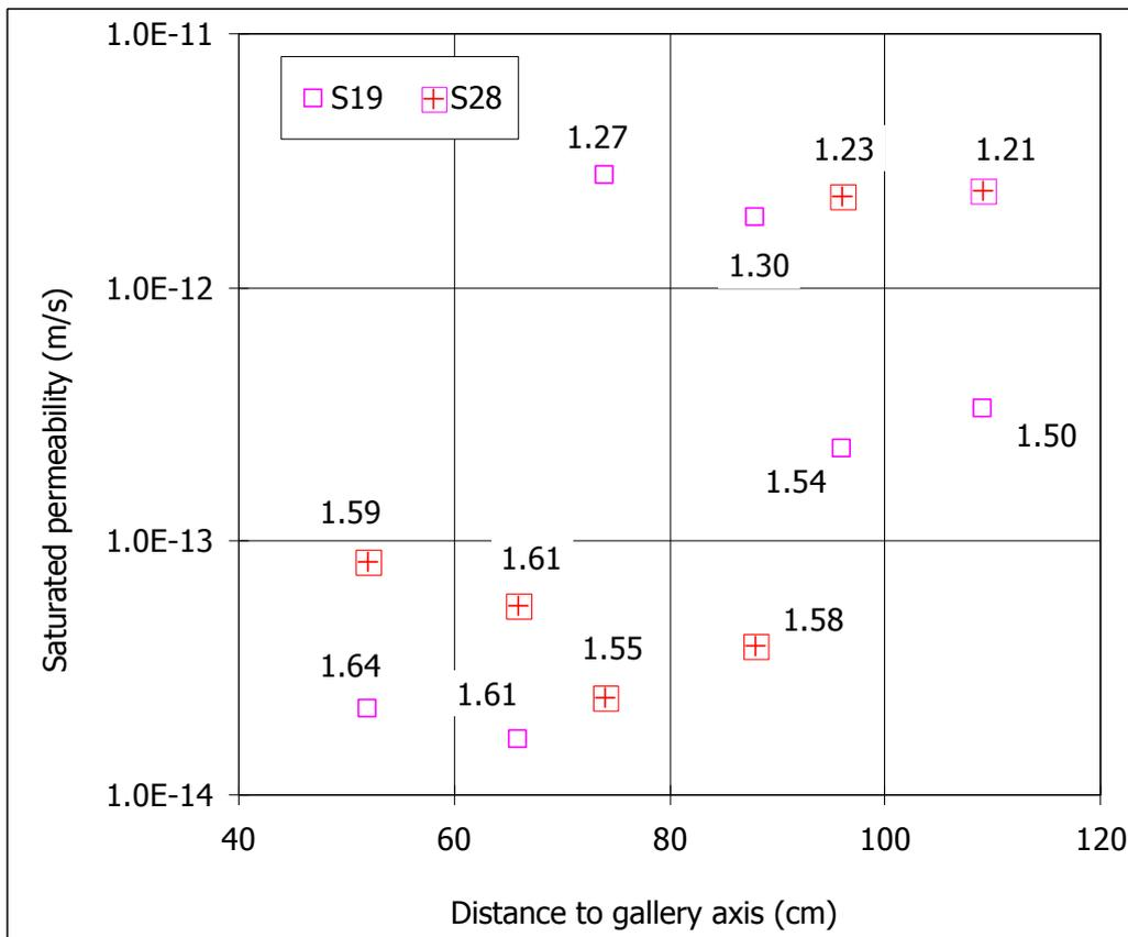
**Figure 27: Hydraulic conductivity of samples from sections S19 and S28 (the dry density of the samples is indicated in g/cm<sup>3</sup>)**
