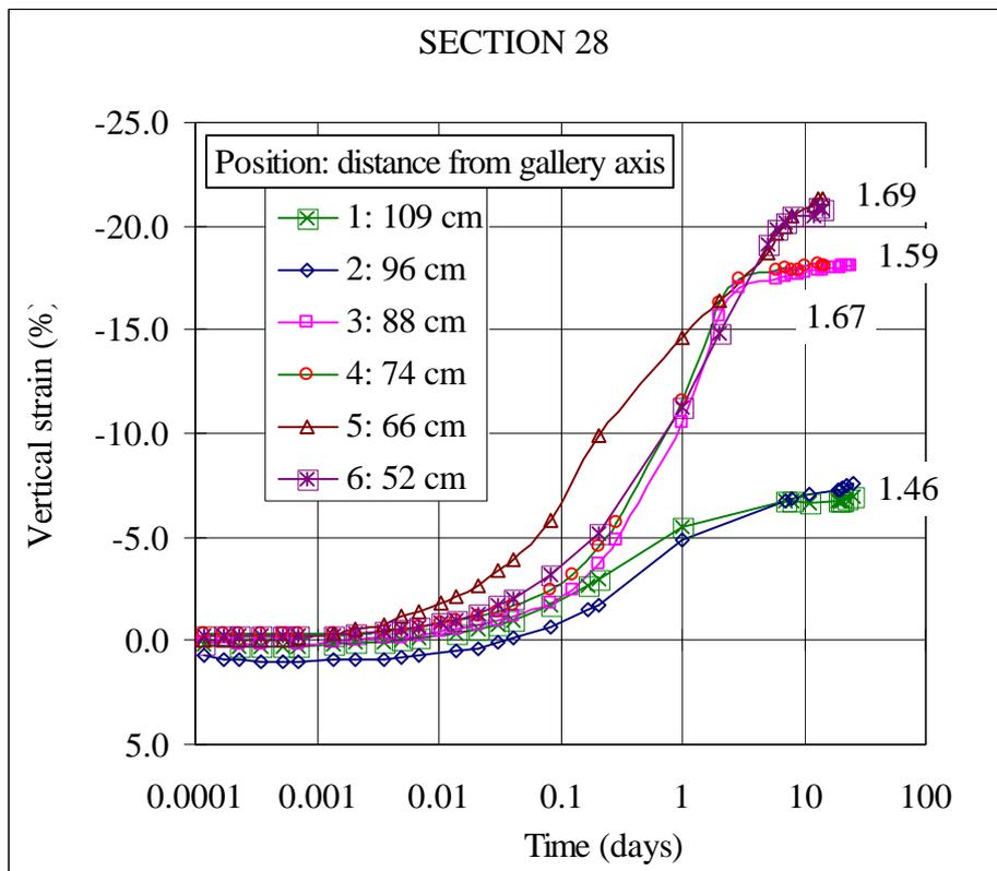
**Figure 32: Evolution of vertical strain during saturation under vertical load 0.5 MPa for samples from section S28 (the initial dry density of the samples is indicated in  $\text{g/cm}^3$ )**
