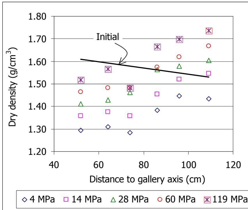
**Figure 18: Dry densities reached under different suctions for samples from section S31**
