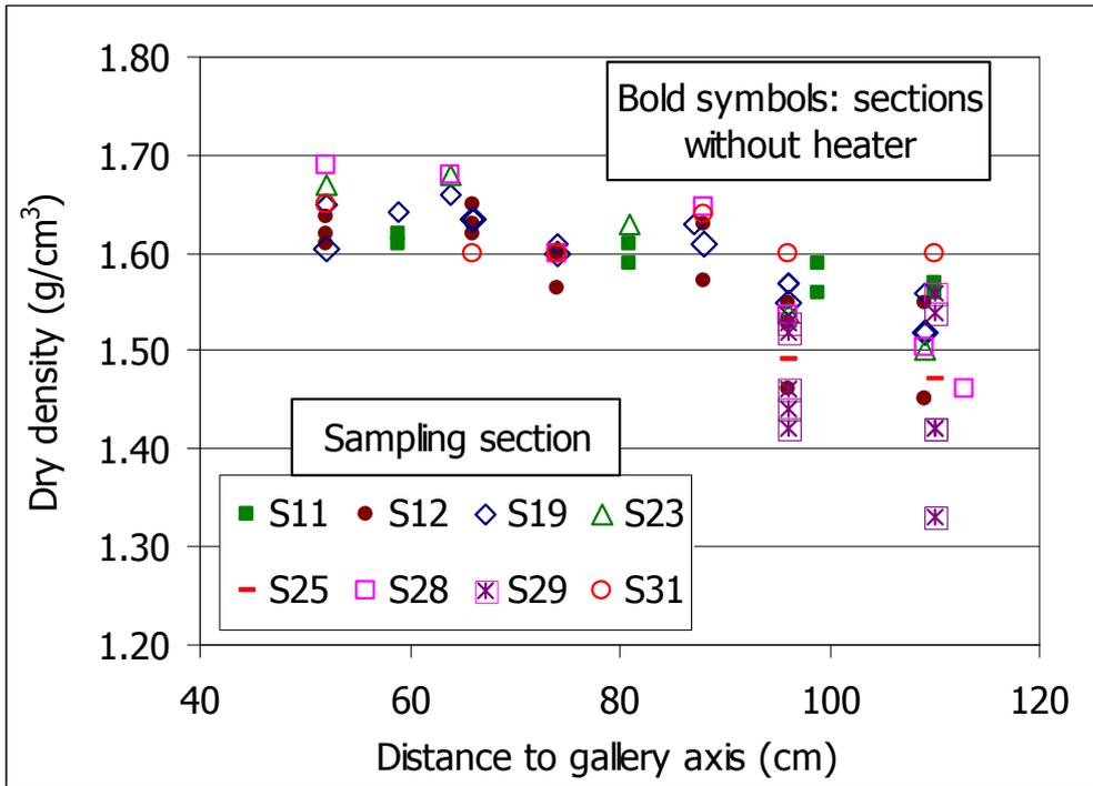
Figure 11: Dry densities measured along radius of different sections
