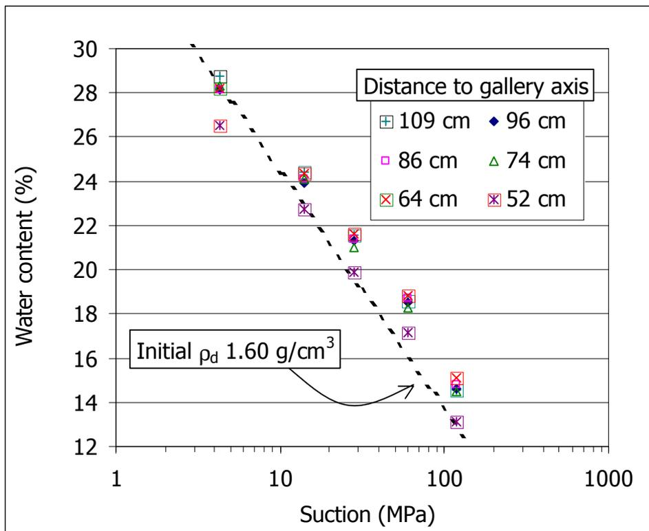
Figure 20: Evolution of water content in a drying path for samples from section S31. The line correspond to untreated FEBEX bentonite in a wetting path (obtained with equation [1])
