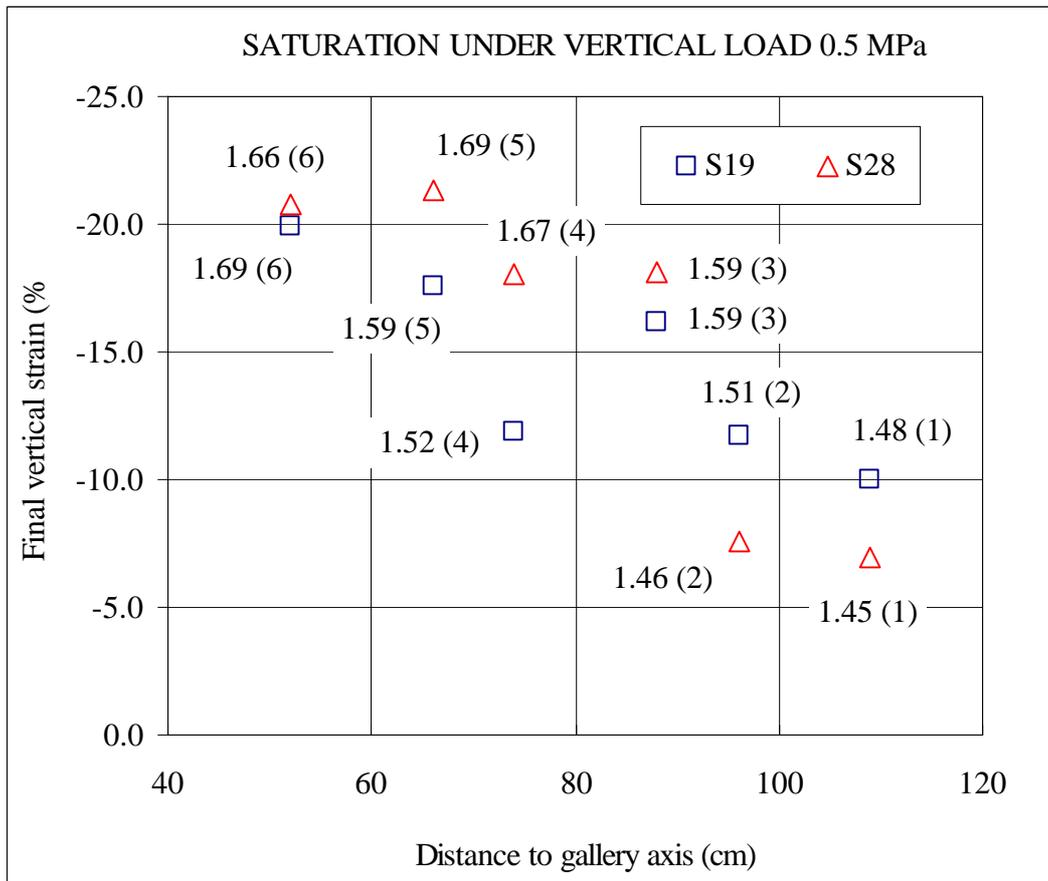
**Figure 30: Vertical strain after saturation under 0.5 MPa of samples from sections S19 and S28 (the initial dry density of the samples is indicated in g/cm<sup>3</sup> and their position by correlative numbers from 1 –close to the gallery wall– to 6 –close to the heater–)**
