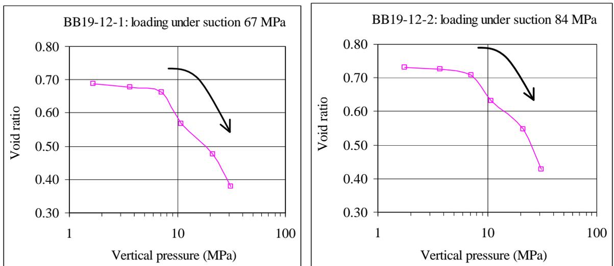
**Figure 44: Oedometric curves of the tests performed in samples from block BB19-12**
