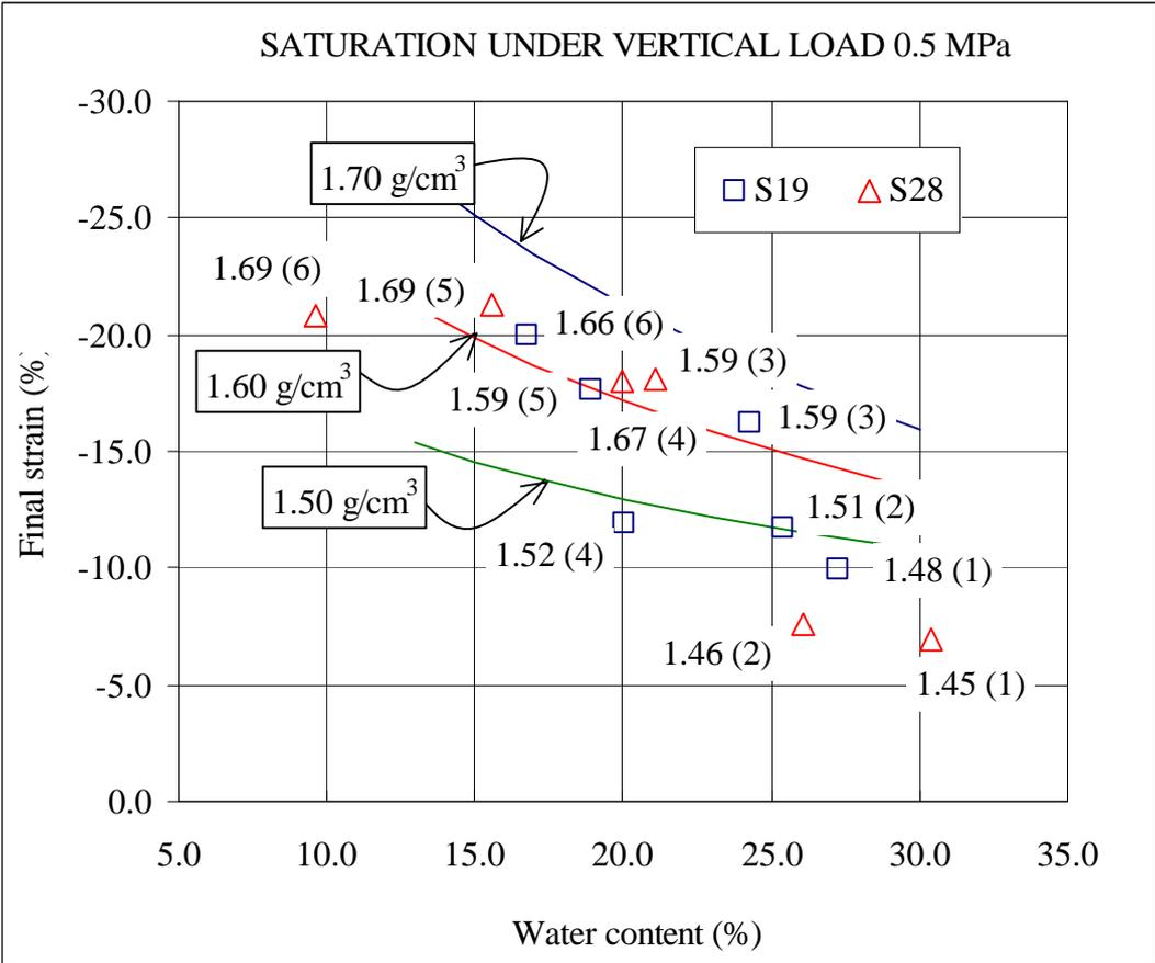
**Figure 33: Final strain reached in soaking tests under a vertical pressure of 0.5 MPa for samples of sections 19 and 28. The lines correspond to the empirical fittings obtained with equation [5] (the initial dry density of the samples is indicated in  $\text{g/cm}^3$  and their positions with correlative numbers from 1 –closest to gallery wall– to 6 –closest to heater–)**
