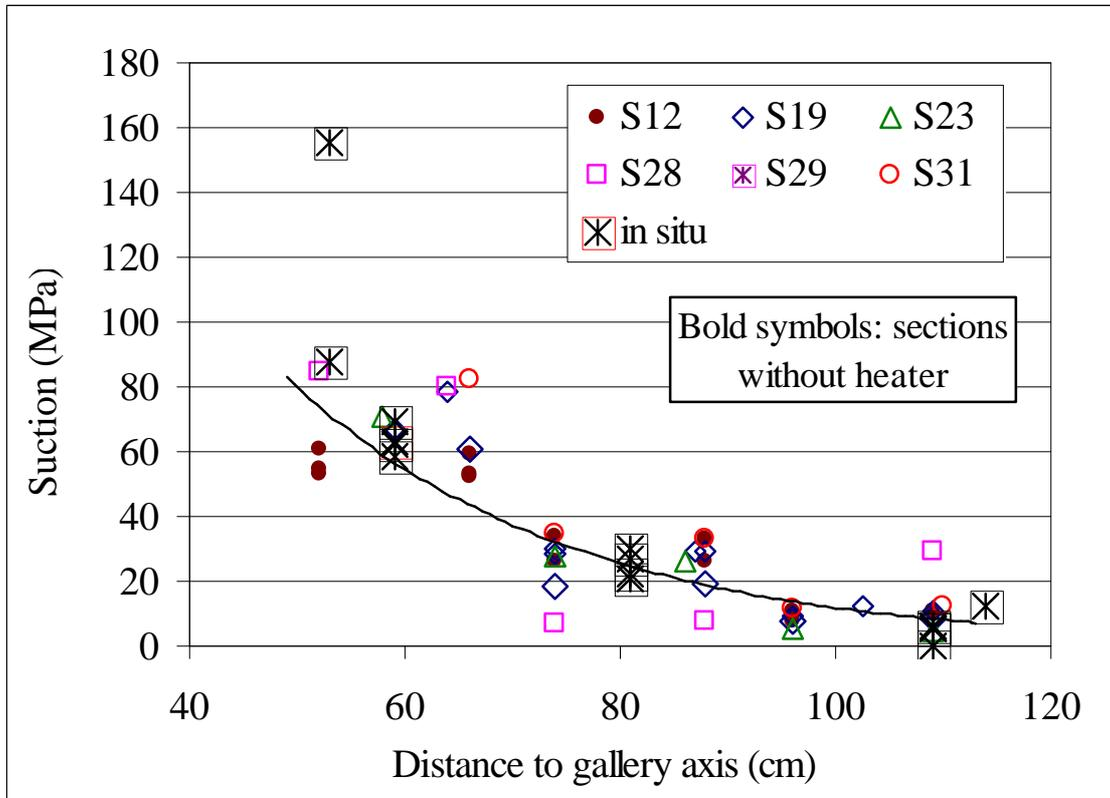
**Figure 22: Suction values measured with capacitive sensors *in situ* before dismantling (instrumented sections C (S11), E1 (S21) and F1 (S25)) and in laboratory. The line is a fitting for all the laboratory measurements**
