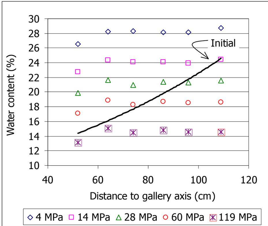
Figure 16: Water contents reached under different suctions for samples from section S31
