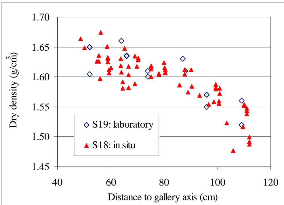
Figure 12: Comparison of dry densities measured *in situ* (UPC) and in laboratory (CIEMAT) in two adjacent sections
