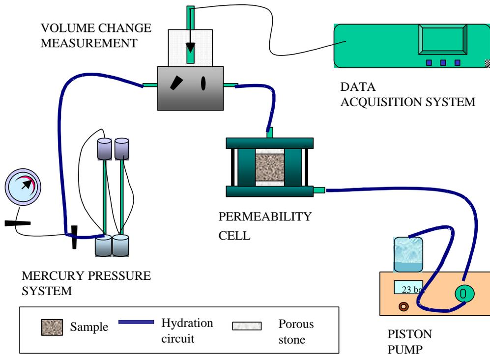
**Figure 26: Schematic representation of hydraulic conductivity measuring assembly for expansive soils**
