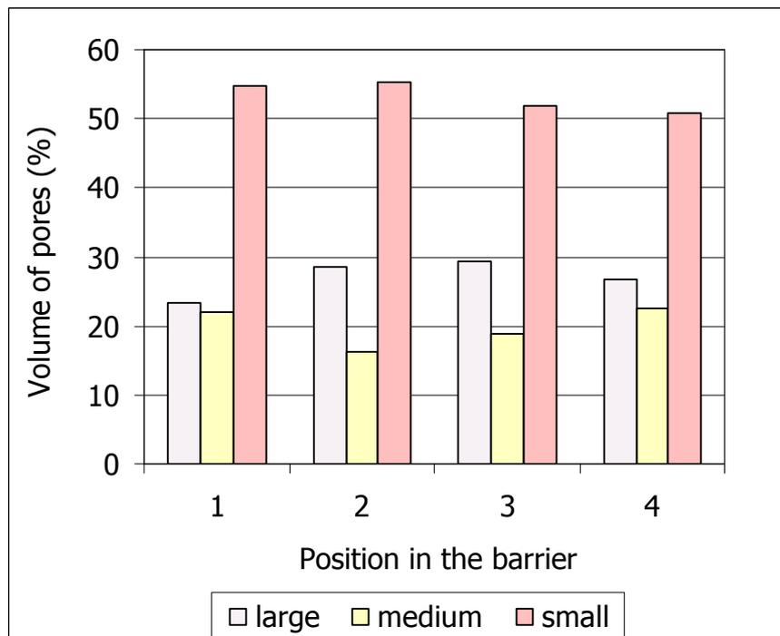
**Figure 25: Distribution of large (> 6 μm), medium (between 6 and 0.15 μm) and small (between 0.15 and 0.006 μm) pores in the untreated bentonite compacted at 1.68 g/cm<sup>3</sup> with hygroscopic water content (1), and external (2), intermediate (3) and inner (4) rings of the clay barrier, obtained by mercury intrusion**
