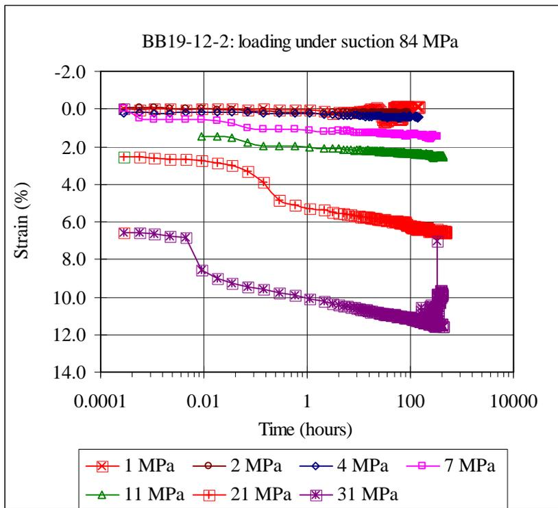
**Figure 41: Evolution of strain during the different steps of the process of loading under suction 84 MPa for sample BB19-12A-2**
