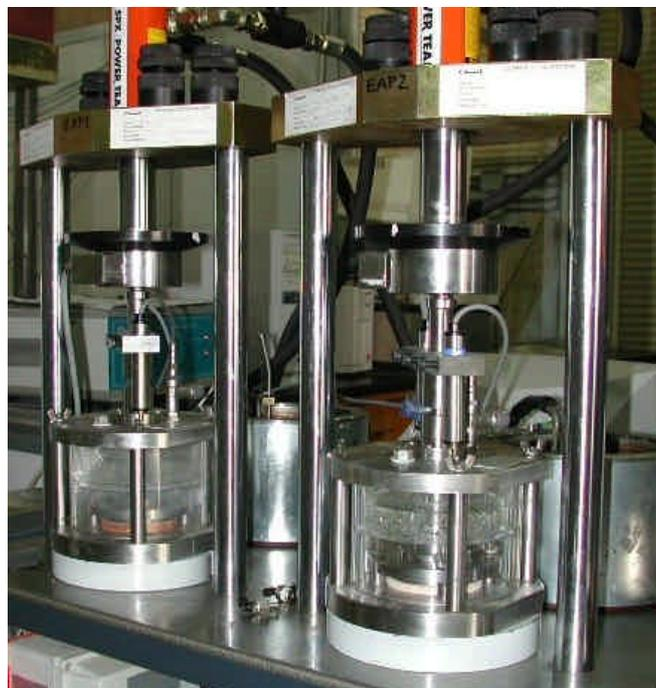
**Figure 35: Suction controlled oedometer cells installed in the frames to perform high pressure consolidation tests**
