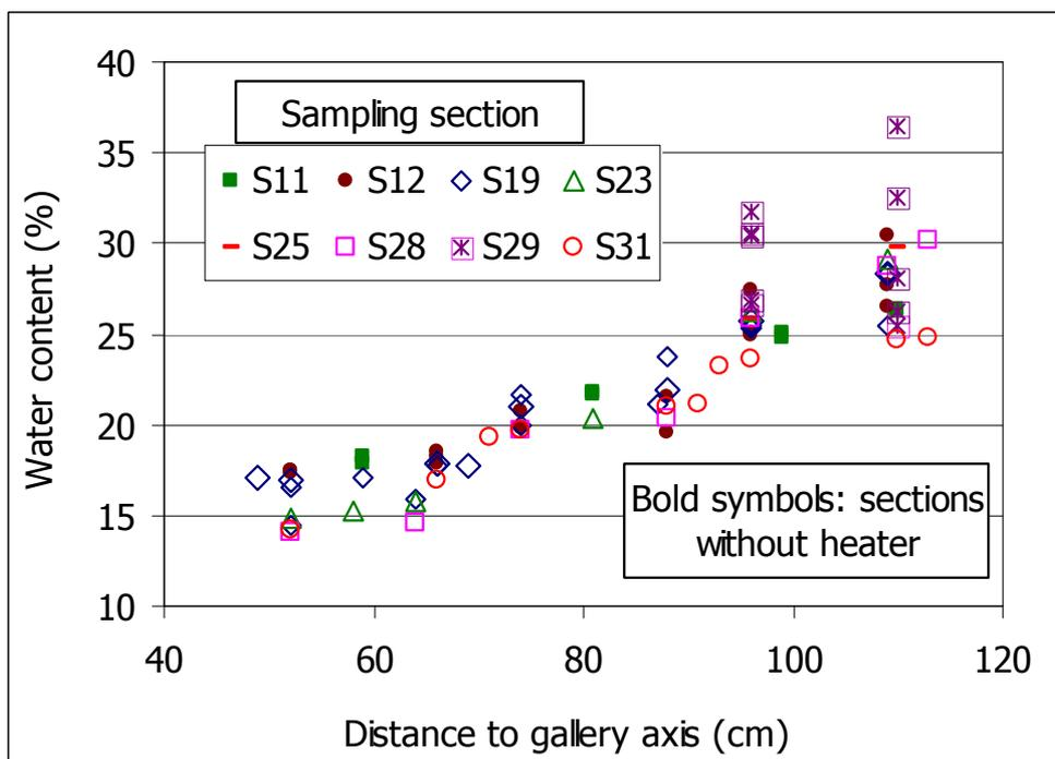
**Figure 9: Water contents measured along radius of different sections**
