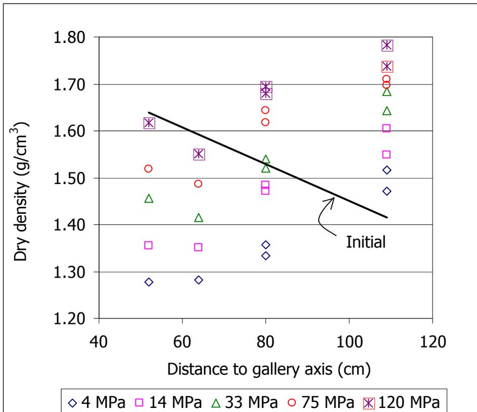
Figure 17: Dry densities reached under different suctions for samples from section S23
