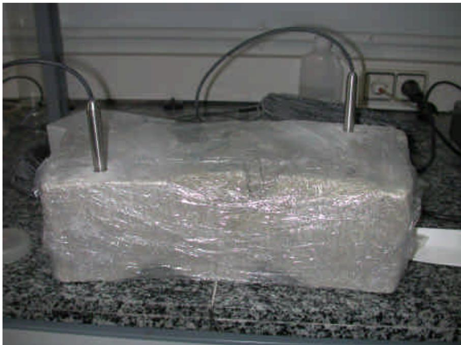
**Figure 21: Capacitive sensors installed in two different positions of a block from Grimsel**
