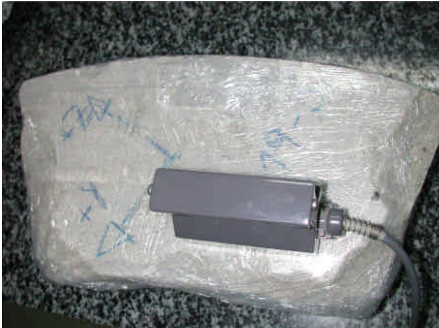
Figure 45: Measurement of superficial thermal conductivity (the plastic foil is removed under the conductivity probe)
