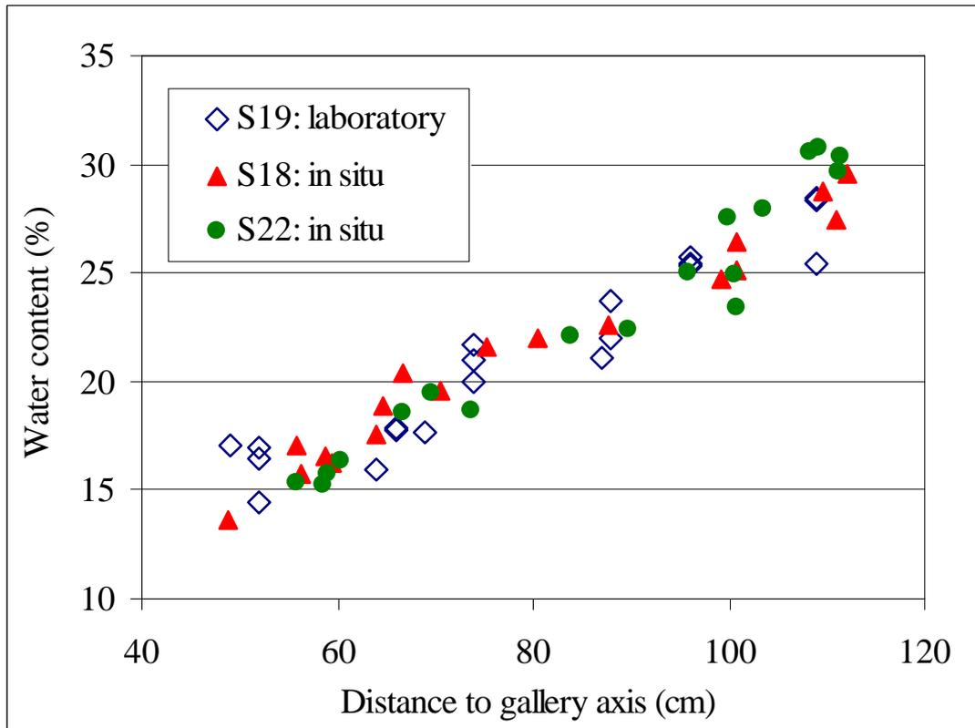
**Figure 10: Comparison of water contents measured *in situ* (UPC) and in laboratory (CIEMAT)**
