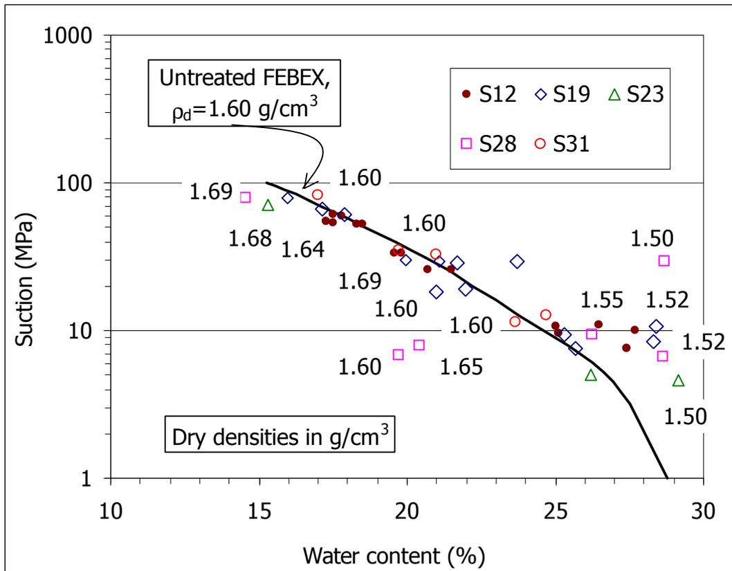
**Figure 23: Retention curve as determined from sensor measurements at laboratory in blocks from different sections(points) and determined in untreated FEBEX samples by control of relative humidity at constant volume (line)**
