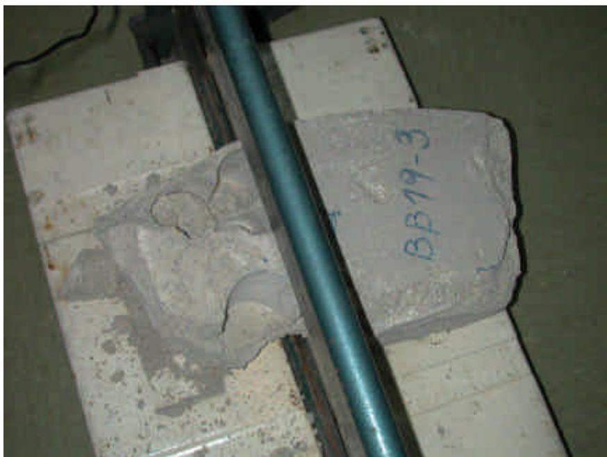
**Figure 6: Sectioning of a block for THM (left) and THG determinations (right)**
