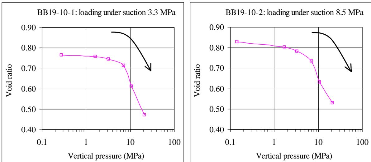
**Figure 42: Oedometric curves of the tests performed in samples from block BB19-10**
