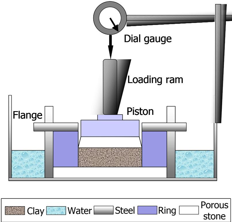
**Figure 29: Schematic cross section of an oedometric cell**
