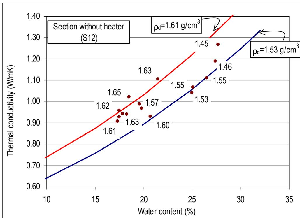
Figure 48: Thermal conductivity values measured in blocks from section S12 (dry density indicated in  $\text{g/cm}^3$ ) and theoretical fittings obtained with Equation 6
