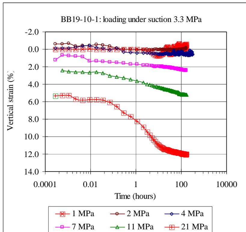
**Figure 36: Evolution of strain during the different steps of the process of loading under suction 3 MPa for sample BB19-10A-1**
