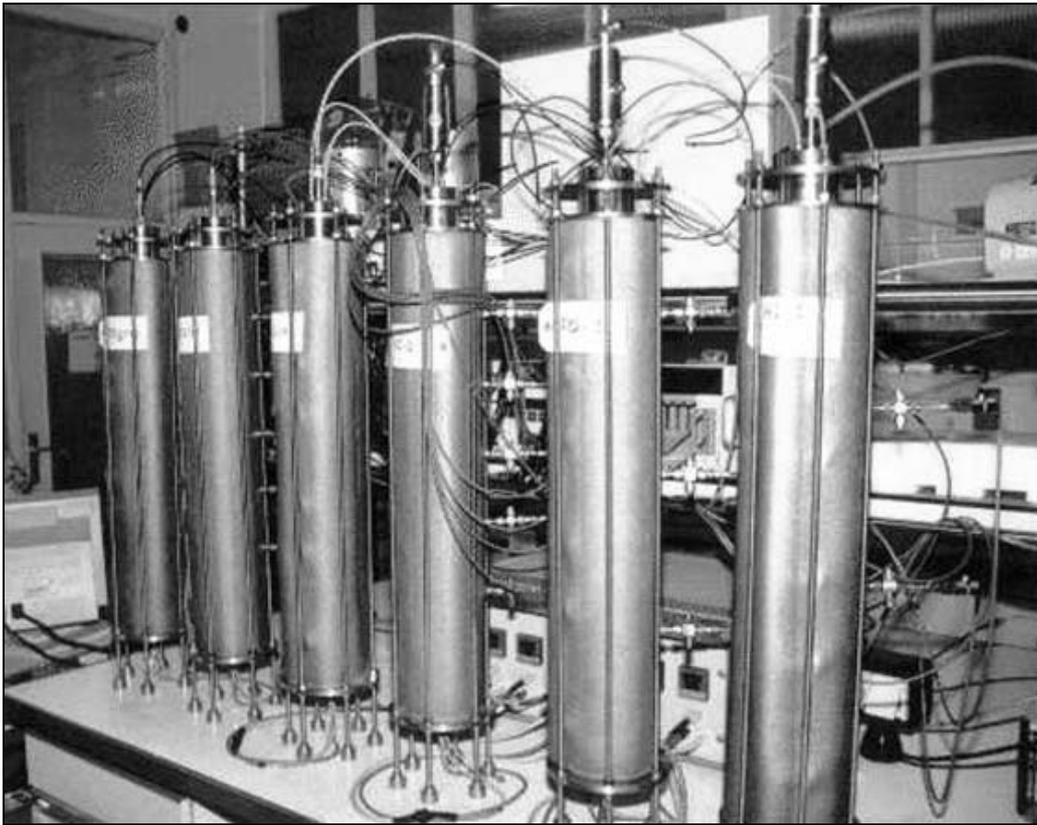
**Figure 29: Experimental set-up for the thermo-hydraulic tests (CIEMAT)**
