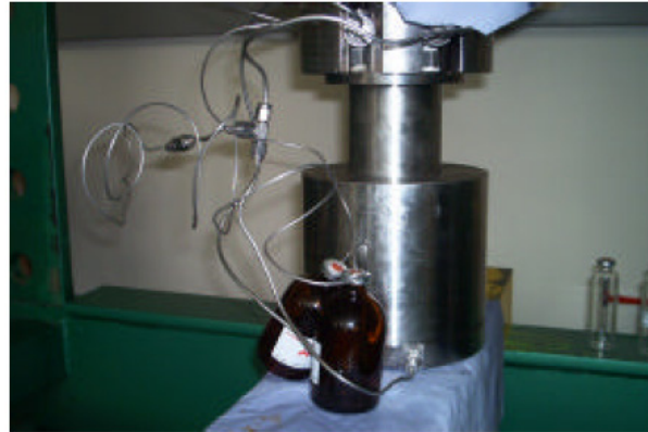
Figure A- 19. Set-up for the extraction of pore water by mechanical squeezing of clay cores. Boom Clay pore water analysis, 30-35 MPa, 40-50 mL water, 700 g sample ( 8 cm \phi /10 cm high), 1 week operation. De Craen et al. (2004)
