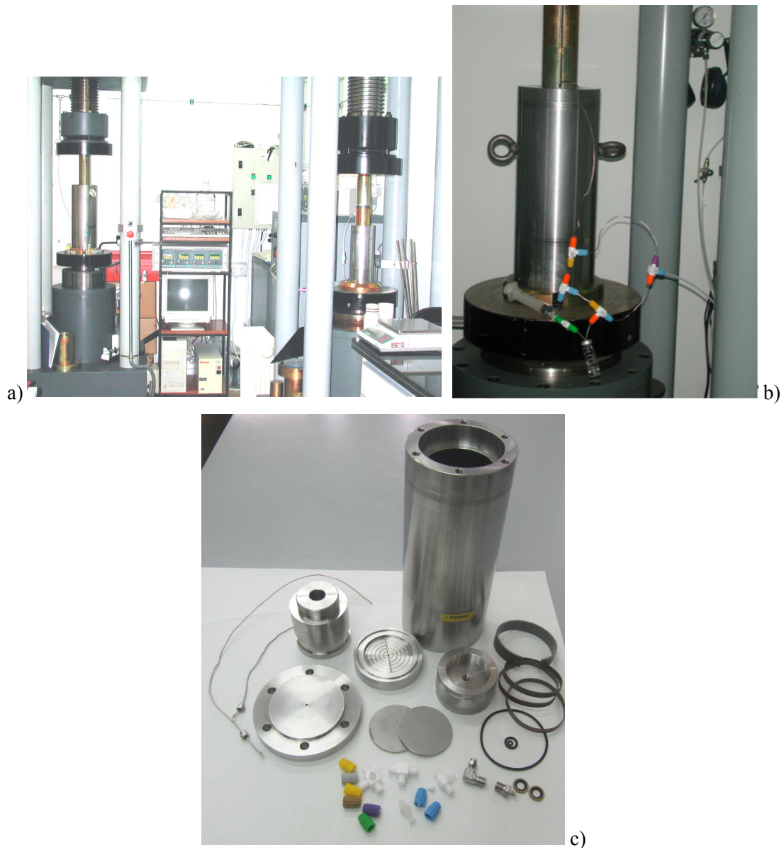
Figure 4. a) Squeezed water extraction apparatus used at CIEMAT; b) Flushing of the squeezing cell and the sampling vial with argon gas prior to the squeezing test; c) pieces of the squeezer
