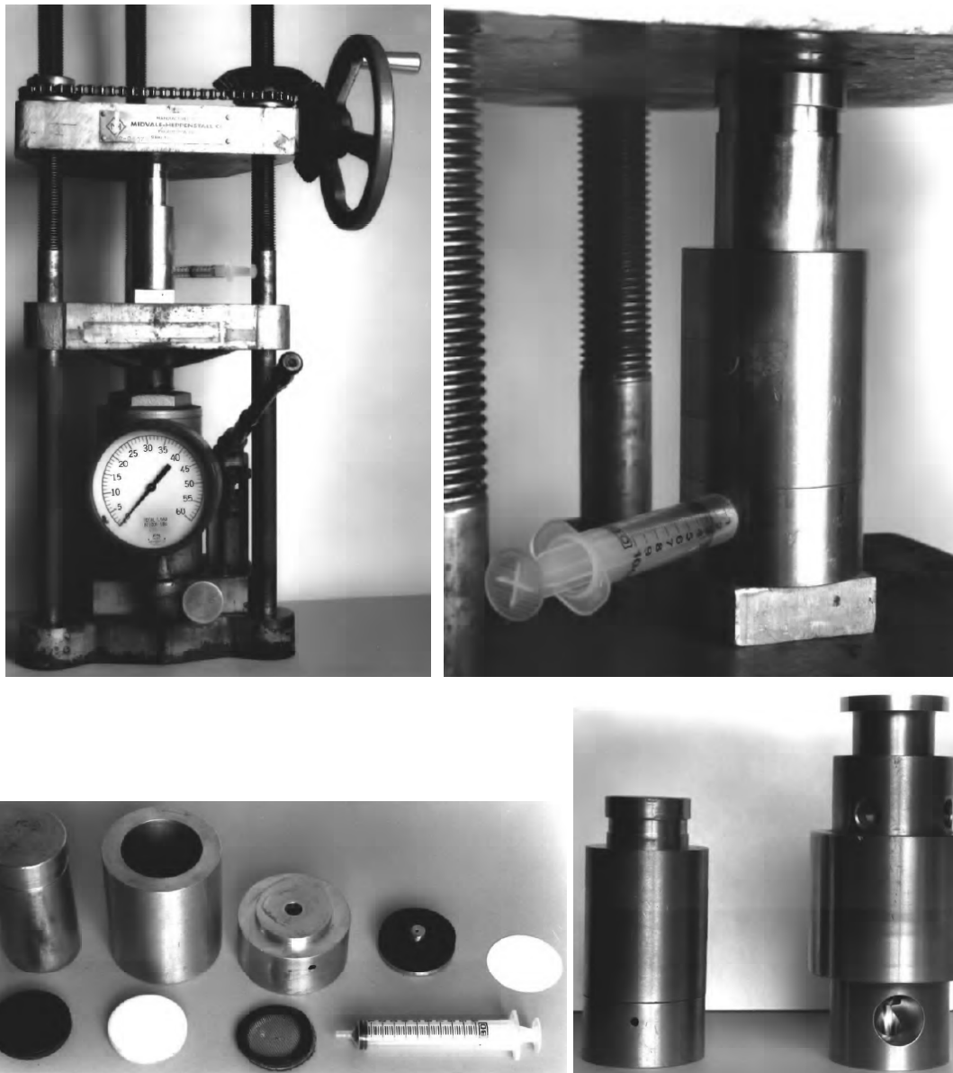
Figure A- 13. A) Hydraulic squeezer set-up for operation used during the Deep Sea Drilling Project, B) Squeezer capsule, disposable syringe and spacer block positioned, C) Squeezer capsule components and accessory parts accompanied by three compressed sediment discs, and D) Stainless steel squeezer capsules used to extract pore fluid from sediments. Left: model A (smallest capsule) used on stiff fine-grained or coarse-grained sediments. Right: model B (largest capsule) used on softer finer-grained sediments. 34-138 MPa, 10-50 cm 3 sample, 10-50 mL water, 10 min. operation. Manheim et al. (1994)
