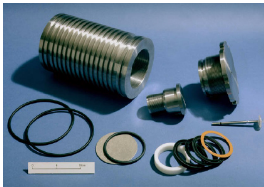
Figure A- 16. Squeezing apparatus and clay squeezing cell, designed and manufactured by R&D Workshop, BGS Keyworth. Entwistle and Reeder (1993), Di Bonito et al. (2008)
