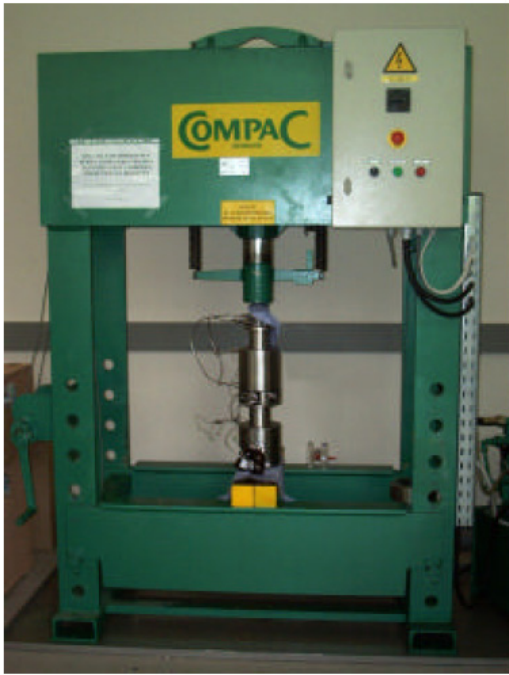
Figure A- 19. Set-up for the extraction of pore water by mechanical squeezing of clay cores. Boom Clay pore water analysis, 30-35 MPa, 40-50 mL water, 700 g sample ( 8 cm \phi /10 cm high), 1 week operation. De Craen et al. (2004)
