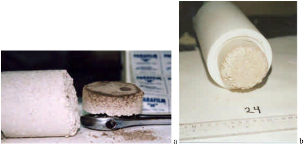
Figure 16: Appearance of the bentonite in contact with the heater in test HI1 (a) and FQ2 (b)
