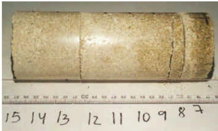
Figure 17: Appearance of a fragment of the bentonite column of test FQ2 upon extraction and establishment of sampling sections
