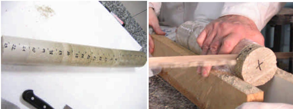
**Figure 4: Establishment of sections along the bentonite and separation by sawing (test CG3)**
