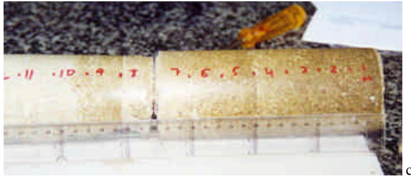
**Figure 14: Final appearance of parts of the bentonite columns in tests HI1/2 (a), HI1 (b) and HI2 (c)**
