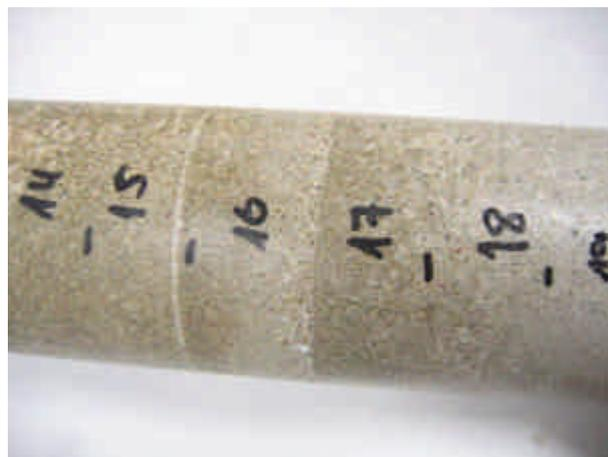
**Figure 15: Appearance of the contact between blocks 4 and 5 (sections 16 and 17) at the end of test CG3**
