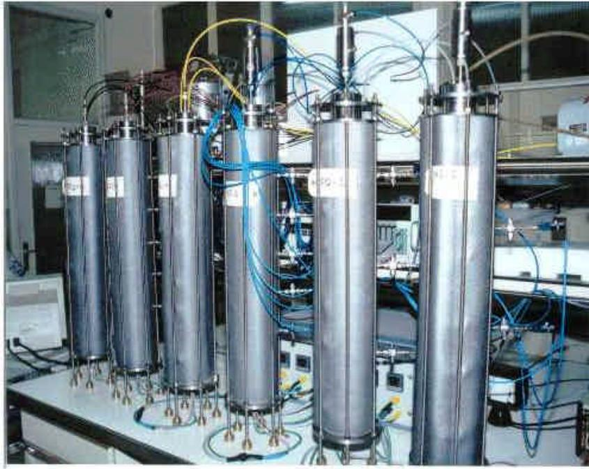
**Figure 3: Infiltration cells in operation**
