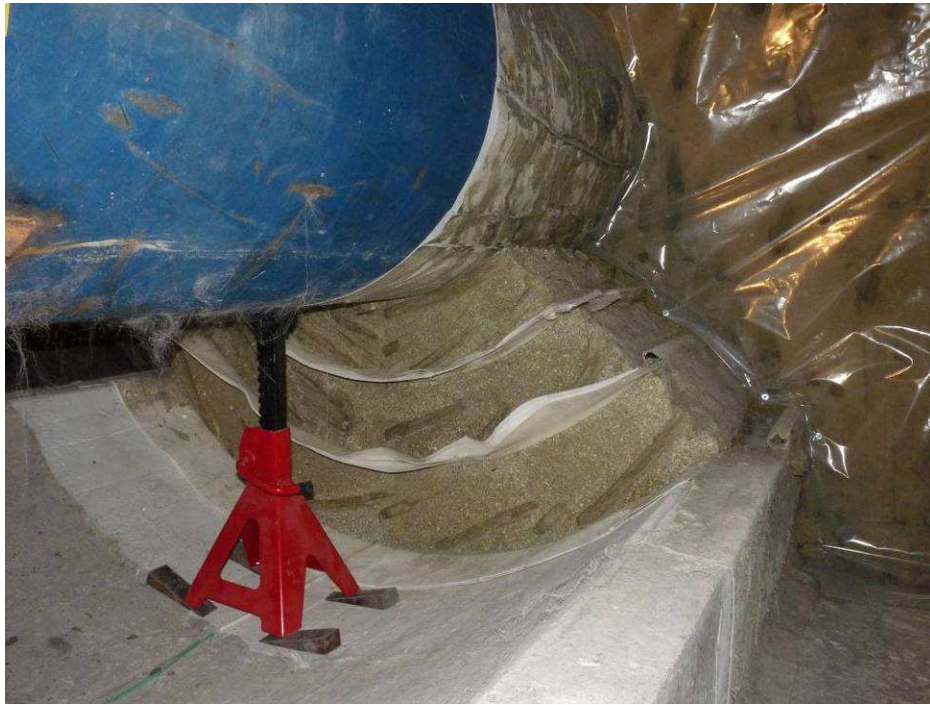
Figure 32: Blocks and bentonite left for demonstrator
