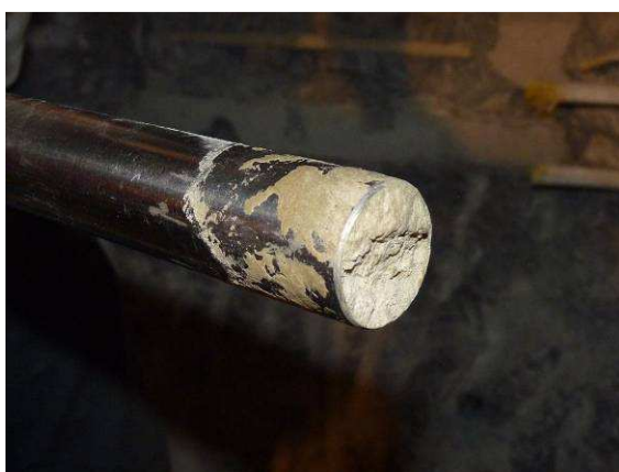
Bentonite sample inside the pipe
