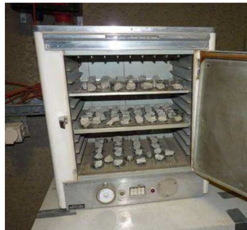
Drying of the samples in the oven
