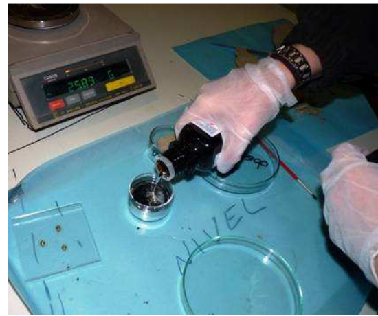
Use of mercury to determine the volume of the subsamples
