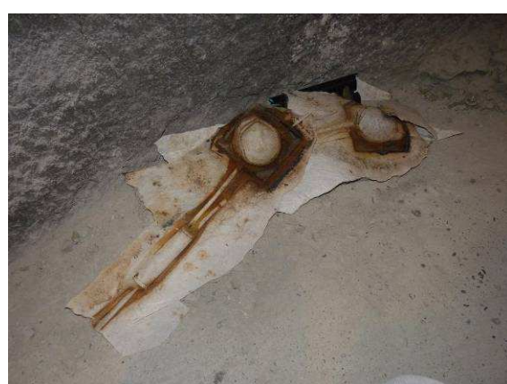
Geotextile covering total pressure cells
