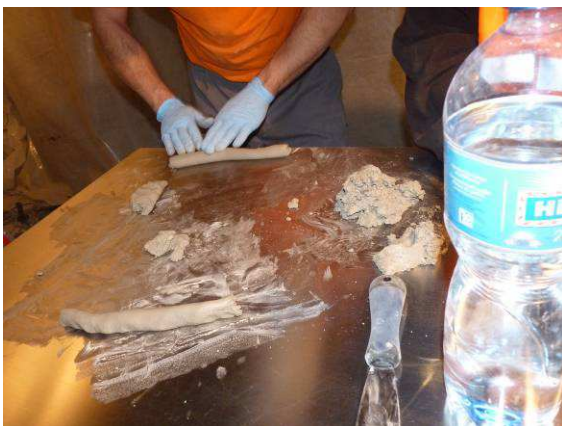
Preparation of the solid expansive cement
