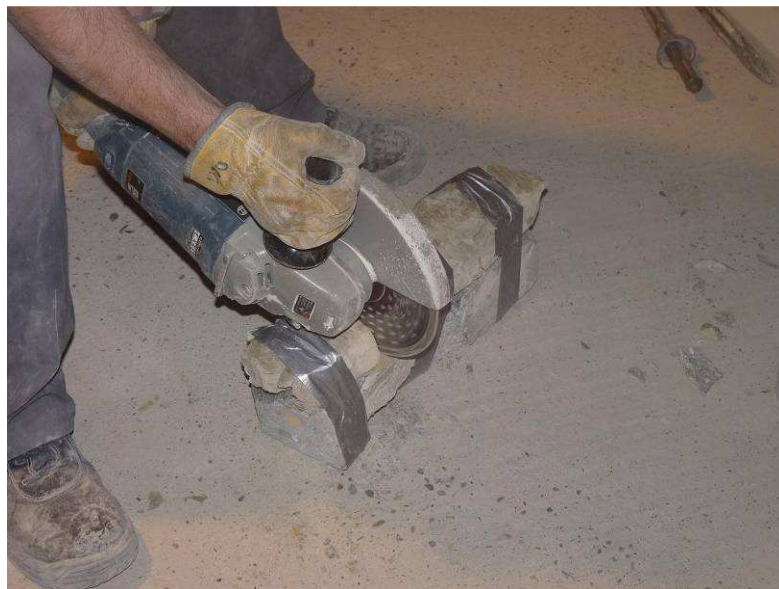
Preparing concrete/bentonite interface samples by cutting them
