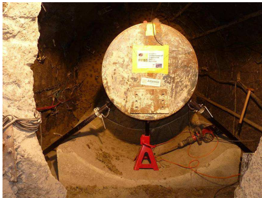
Figure 28: Sawhorse support for canister
