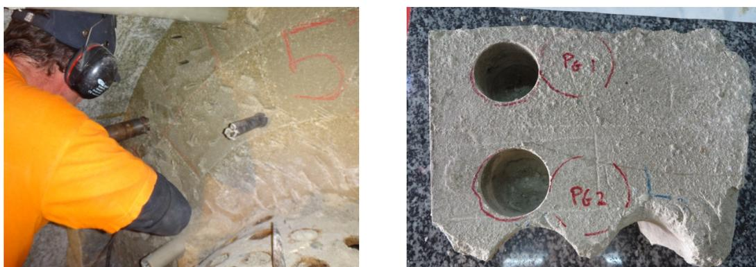
Fig. 28: Sample drilled on site at the contact between blocks (left) and in the laboratory (right)
