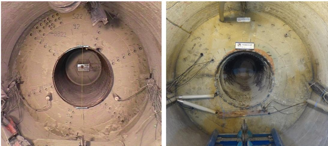
Fig. 5: Appearance of the bentonite barrier after extraction of heater #1 in 2005 and of heater #2 in 2015
