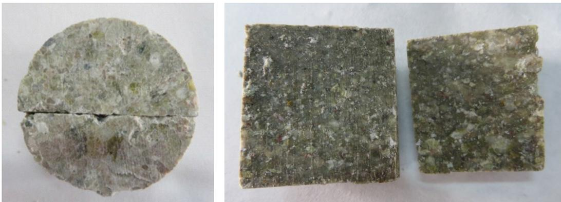
Fig. 30: Appearance of a specimen prepared for gas test with interface between blocks
