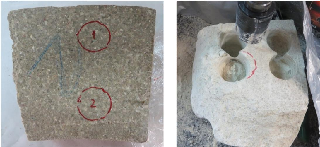
Fig. 21: Location in the blocks of sampling positions for water content and dry density (and most of the other determinations)
