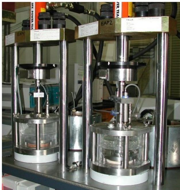
Fig. 37: Suction-controlled oedometer cells installed in the frames to perform high pressure consolidation tests
