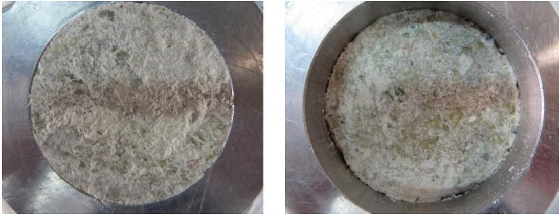
Fig. 34: Appearance of the base and the upper part of a sample inserted in the oedometer ring
