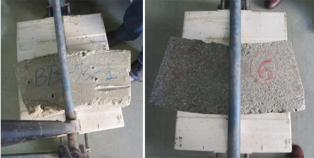
Fig. 15: Sectioning of blocks for THM and THG determinations
