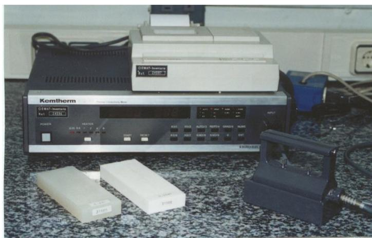
Fig. 18: Kemtherm QTM-D3 conductivity meter with probe and standard plates
