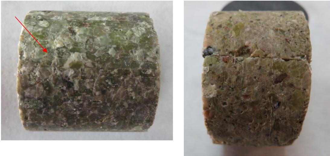
Fig. 92: Interface in a sample from the external ring (indicated by an arrow, BC-44-6) and from the inner ring (BC-44-2)
