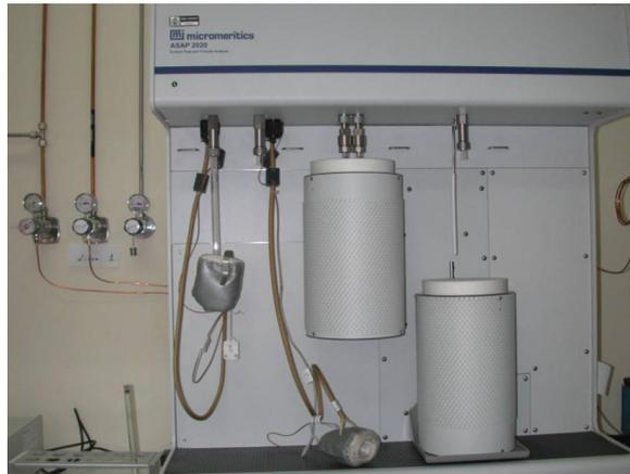
Fig. 23: Equipment used for the determination of  $\text{N}_2$  sorption isotherms (Micromeritics ASAP 2020)
