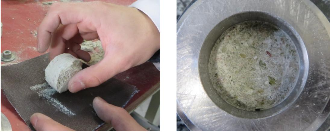
Fig. 38: Preparation of samples for the consolidation tests
