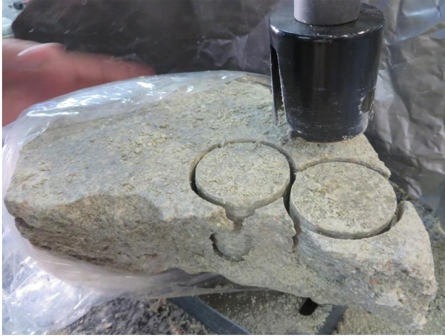
Fig. 26: Drilling of cores to obtain samples for the hydraulic conductivity tests
