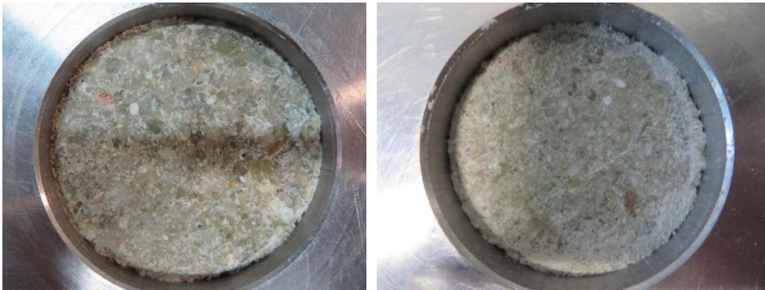
Fig. 27: Appearance of the samples drilled from the blocks inside the permeability cell rings
