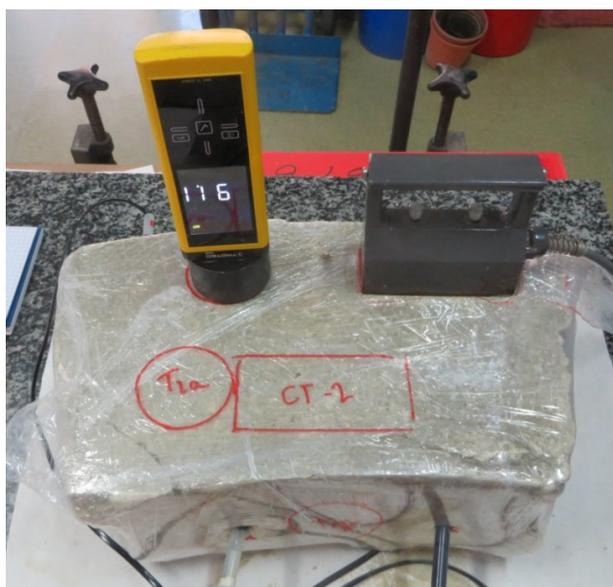
Fig. 14: Measurement of thermal conductivity, relative humidity and moisture before sampling the blocks
