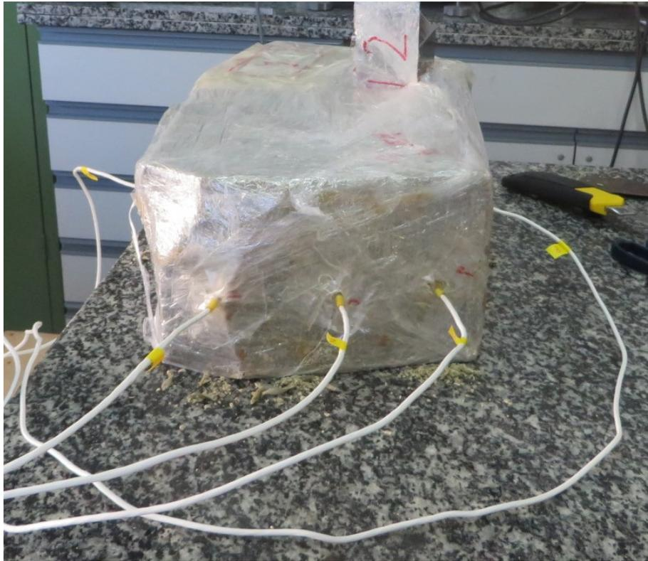
Fig. 20: Psychrometers inserted into a block prior to unpacking
