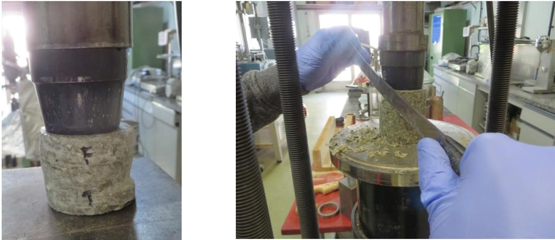
Fig. 29: Sample preparation: adjusting the diameter
