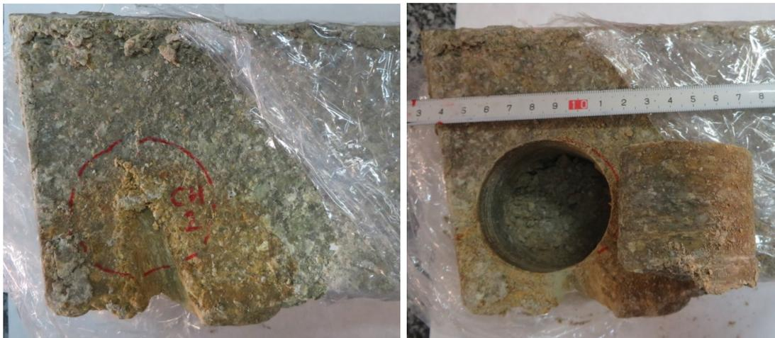
Fig. 122: Drilling of sample BB-59-8-2 in an area affected by the oxidation of an extensometer
