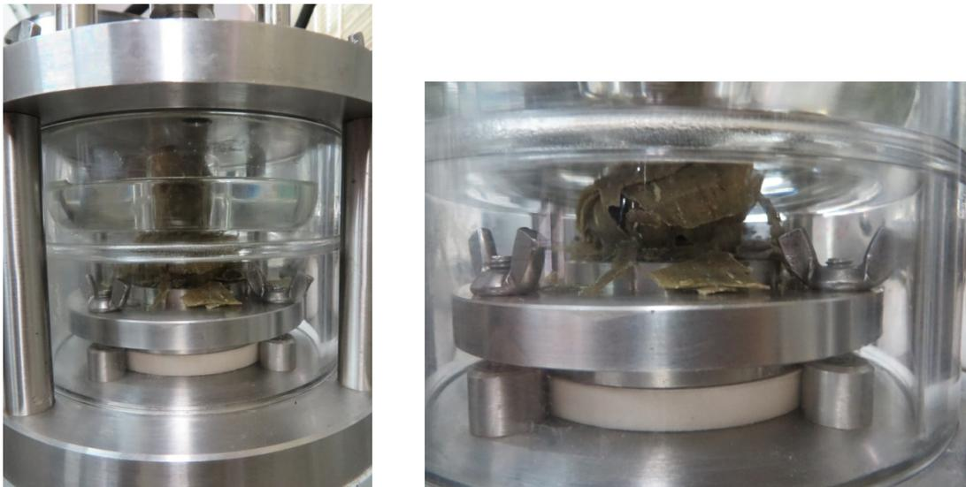
Fig. 131: Sample BB-47-7-2 extruding out of the oedometer ring after loading step at 17 MPa
