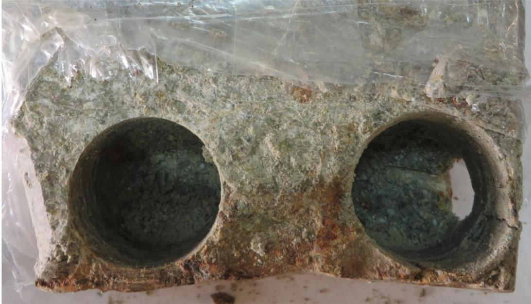
Fig. 121: Location of samples (2a and 2b) drilled close to the liner in block BB-36-3
