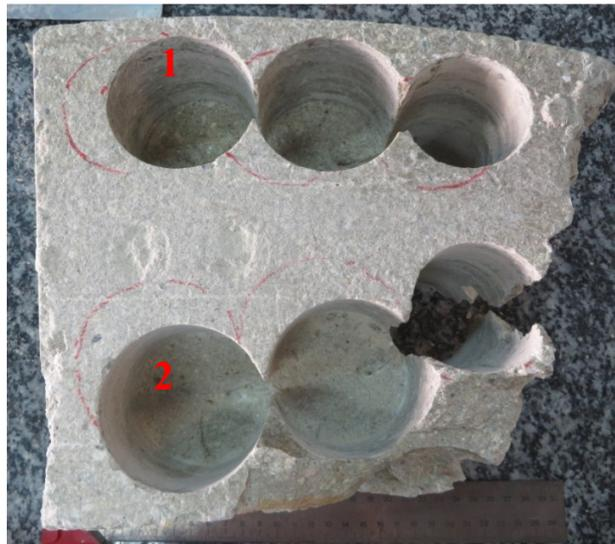
Fig. 16: Drilling of a block to obtain subsamples 1 (closest to the granite) and 2 (closest to the gallery axis) for HM determinations
