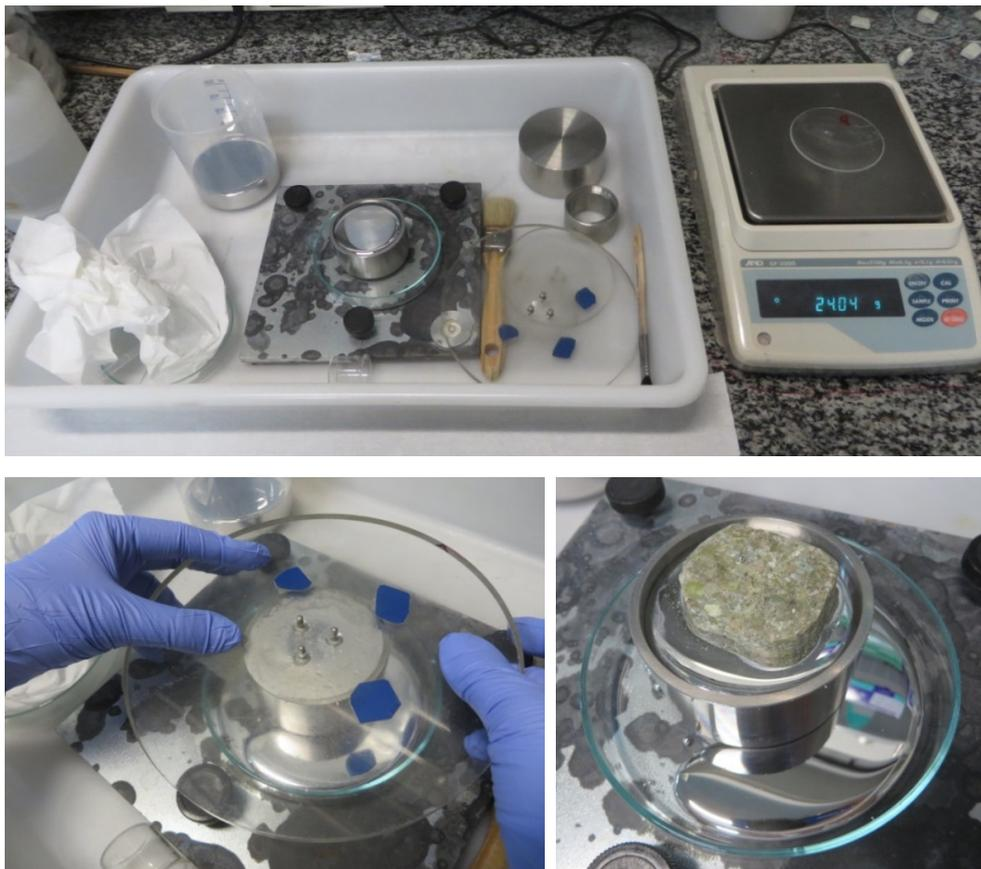
Fig. 22: Determination of sample volume by immersion in mercury
