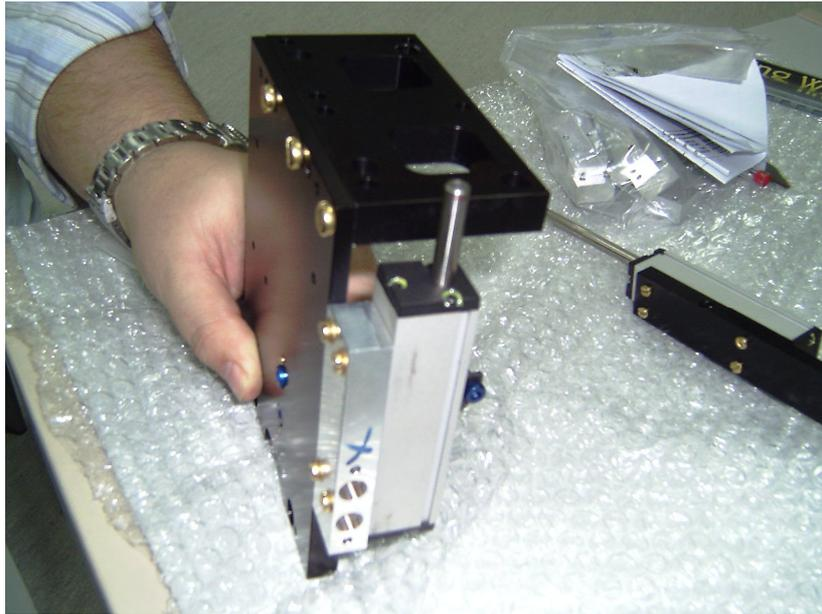
**Fig. 36:** View of the sensor support and attach to the TP for the monitoring of the relative radial distance between the TP and the ME/1/2 chamber.
