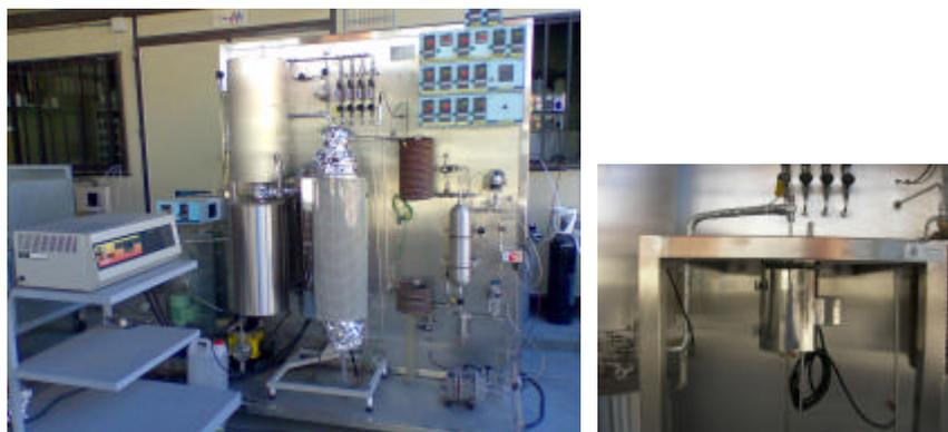
**Fig. 16.** Membrane Reactor bench-scale plant (**left**) oven for pre-commercial membrane installed (**right**) oven for prepared membranes installed
