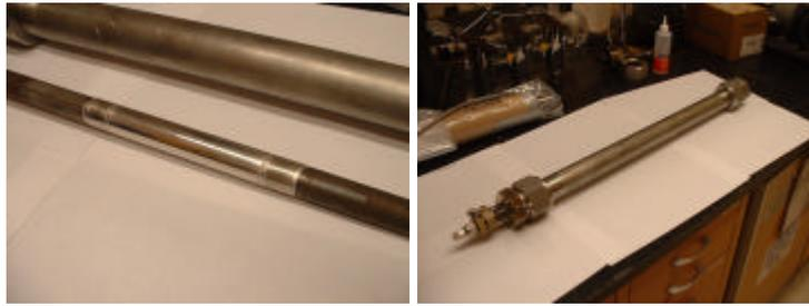
**Fig. 14. (left) Pre-commercial membrane (right) Membrane reactor**
