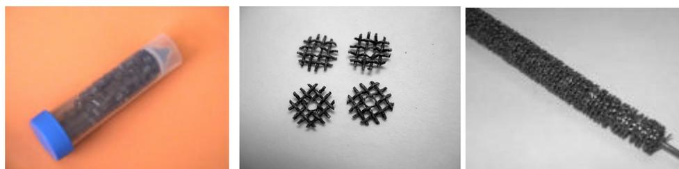
**Fig. 4:** Samples of catalyst used for WGS studies **(left)** Fe-Cr pellets; **(center)** Pt-based sheets; **(right)** Pt-based catalyst as mounted in the reactor
