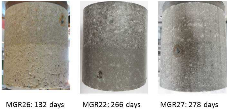
Fig. 8. Appearance of the MGR samples at the end of the tests performed under constant water inflow rate (MGR22, MGR26) and with saturation through the block (MGR27)
