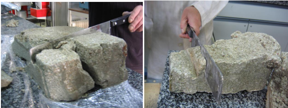
Figure 9: Sectioning of blocks to obtain subsamples
