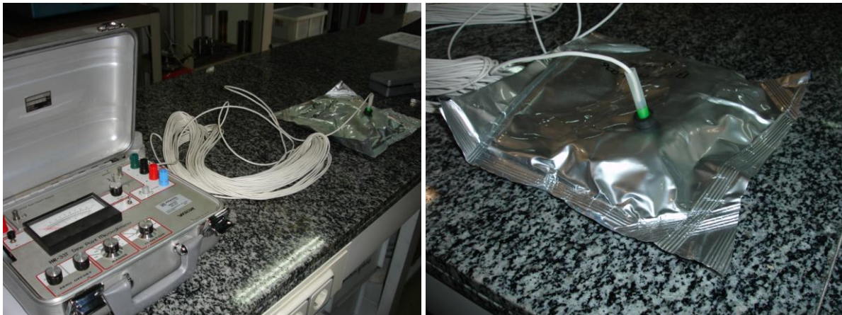
Figure 11: Measurement of relative humidity and temperature with psychrometers
