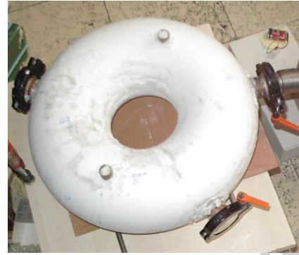
Fig. 8. Finished smoothed and completely circular monolithic frame without grooves.
