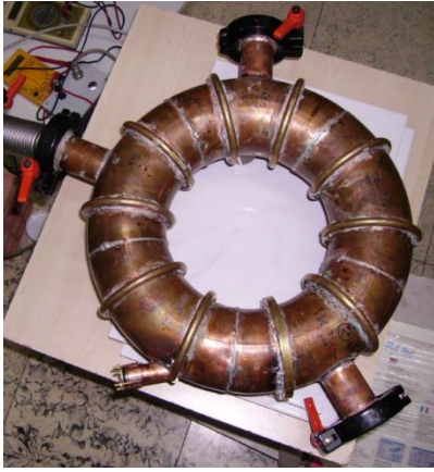
Fig. 6. UST_1 vacuum vessel.
