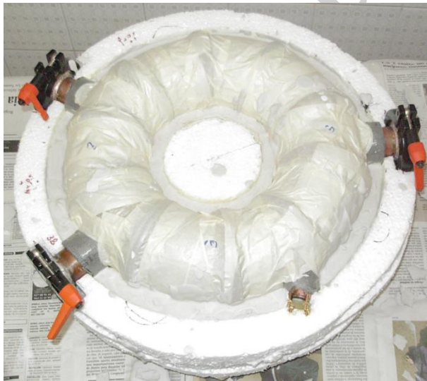
Fig. 7. Expanded polystyrene mould and vacuum vessel covered by a separation layer.
