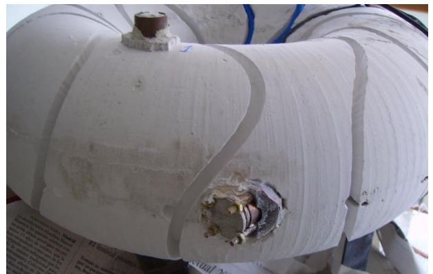
Fig. 9. Monolithic frame and grooves for the coils.
