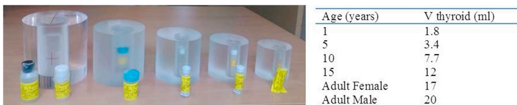
Fig. 1. Neck and vial phantoms with their volumes of ^{131}\text{I} .
