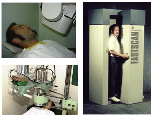
Fig. 1. In vivo measurement of 131 I in thyroid at Whole Body Counter laboratory of CIEMAT.
