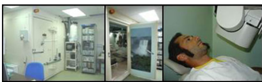
Figure 1. Thyroid monitoring using a LEGe detector inside a shielded room at CIEMAT WBC.
