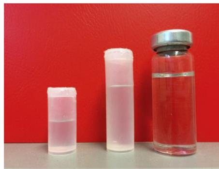
Fig. 2. Vials with a solution of  $^{133}\text{Ba}$  and  $^{137}\text{Cs}$ , representing thyroid sizes for 5 y ( $2 \times 1.6$  ml), 10 y ( $2 \times 3.75$  ml) and adults ( $2 \times 9.5$  ml).
