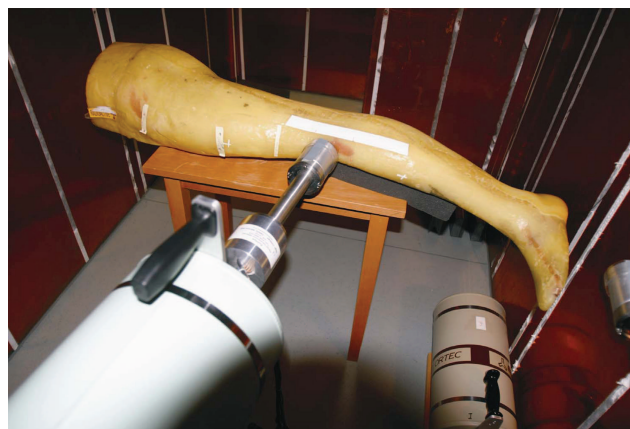
Fig. 1. HMGU's counting chamber that can be used for in vivo counting. In this picture, one detector is being used to measure the ^{241}\text{Am} in the phantom's bone.
