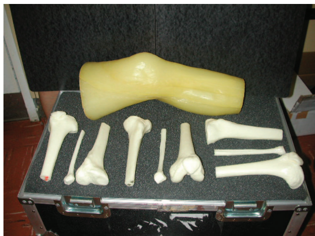
Fig. 2. The commercial knee phantom borrowed from the IAEA showing the insert sets.
