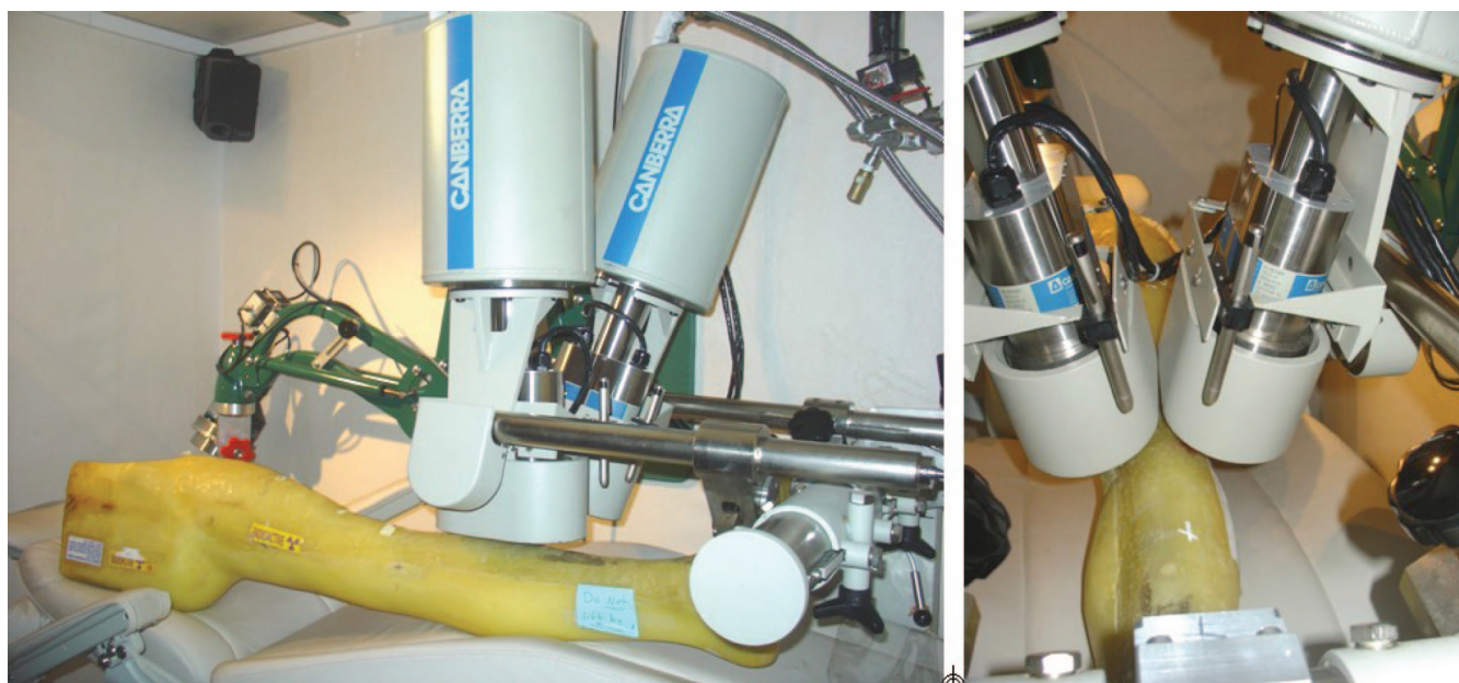
Fig. 6. In vivo monitoring of USTUR leg phantom at CIEMAT: (1) vertical position of two-detector array and (2) wrapping counting geometry of four LEGe detectors.
