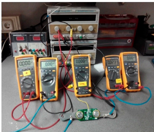
Figure 11. Experimental test to measure the current through the active balance circuit when the voltage in the cell is above 2.6 V.
