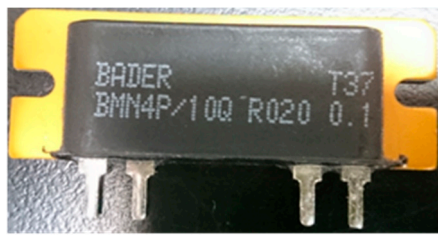
Figure 8. Shunt resistance used in the assays; shunt resistance datasheet.
