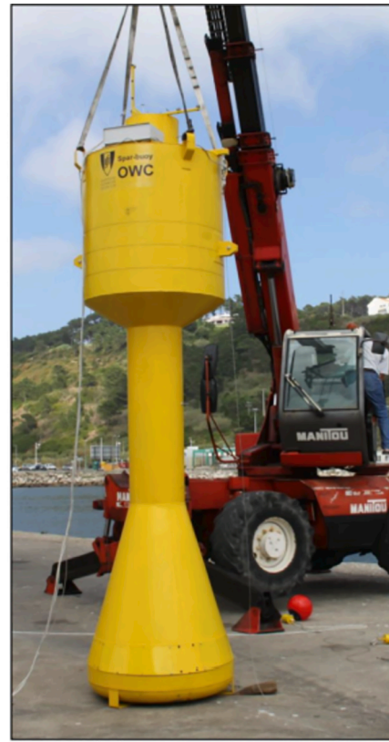
Fig. 1. Scheme (left) and photography (right) of a floating OWC WEC [16].
