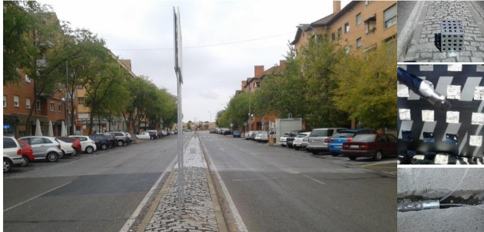
275 Figure 3. Photocatalytic stretch of the Paseo de la Chopera. Sampling points P2 and P3 together with the corresponding 276 booth can be distinguished. Details of a meshed cage, a particulate filter at a sampling point and sampling lines 277 before being buried are also shown.
