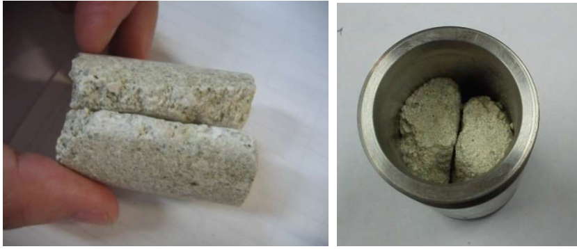
Fig. 3. Appearance of samples prepared for interface testing prior to saturation (sample JB1.6_38)
