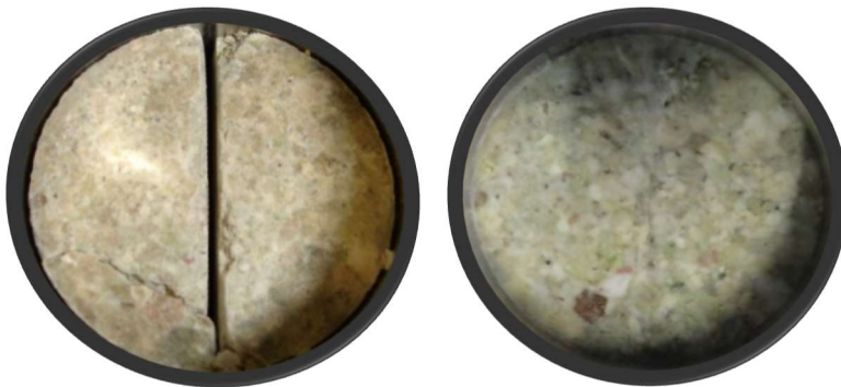
Fig. 16. Appearance of sample JB19_38 inside the cell before starting testing (left) and after saturation in Phase 1 (right)
