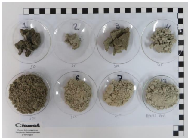
Figure 23 Samples left in the laboratory atmosphere for water content stabilisation
