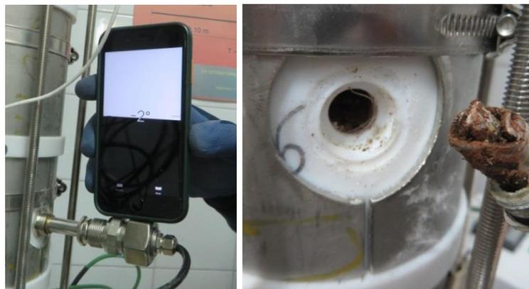
Figure 27 Extraction of sensor RH/T3 and appearance after extraction
