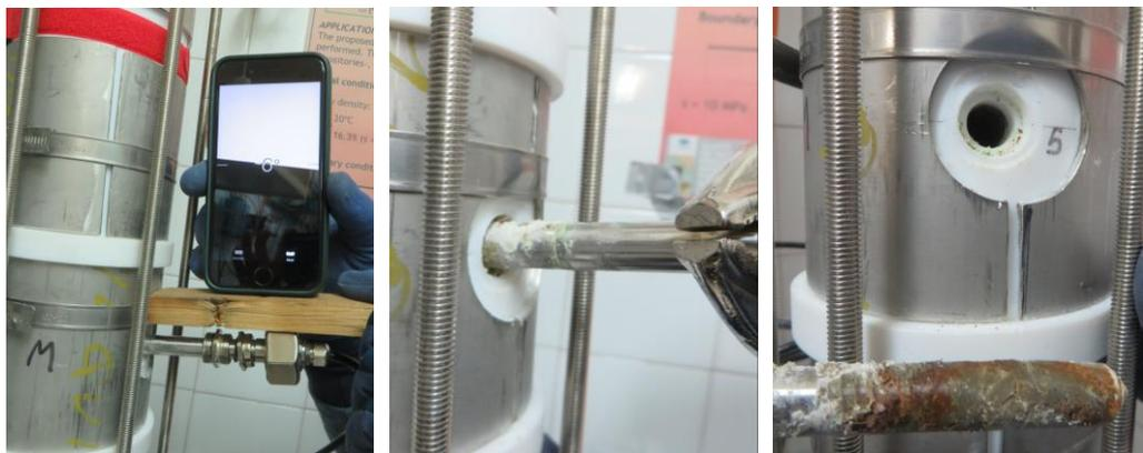
Figure 26 Sequence of extraction of sensor RH/T2
