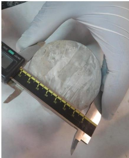
Figure 45 Measurement of diameter in compact samples
