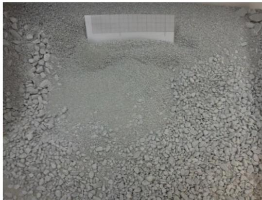
Figure 3 Appearance of the MX-80 bentonite pellets received at CIEMAT
