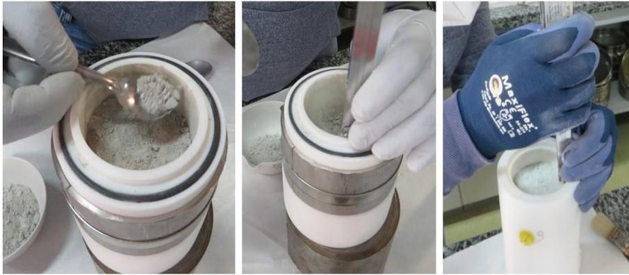
Figure 33 Subsampling of loose sections S25 to S20 and measurement of sampling sections height
