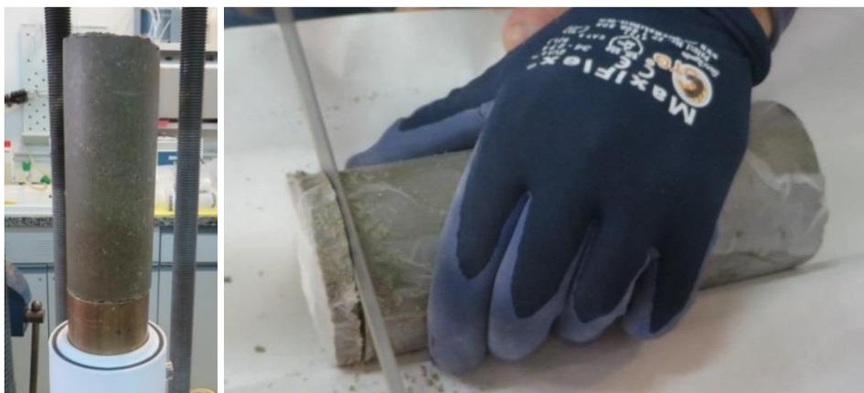
Figure 35 Extraction and sampling of the part of the column corresponding to sections S12 to S2
