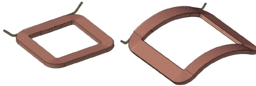
Figure 5. 3D model of corrector coils corresponding to a first triplet magnet (left) and to a second triplet magnet (right).
