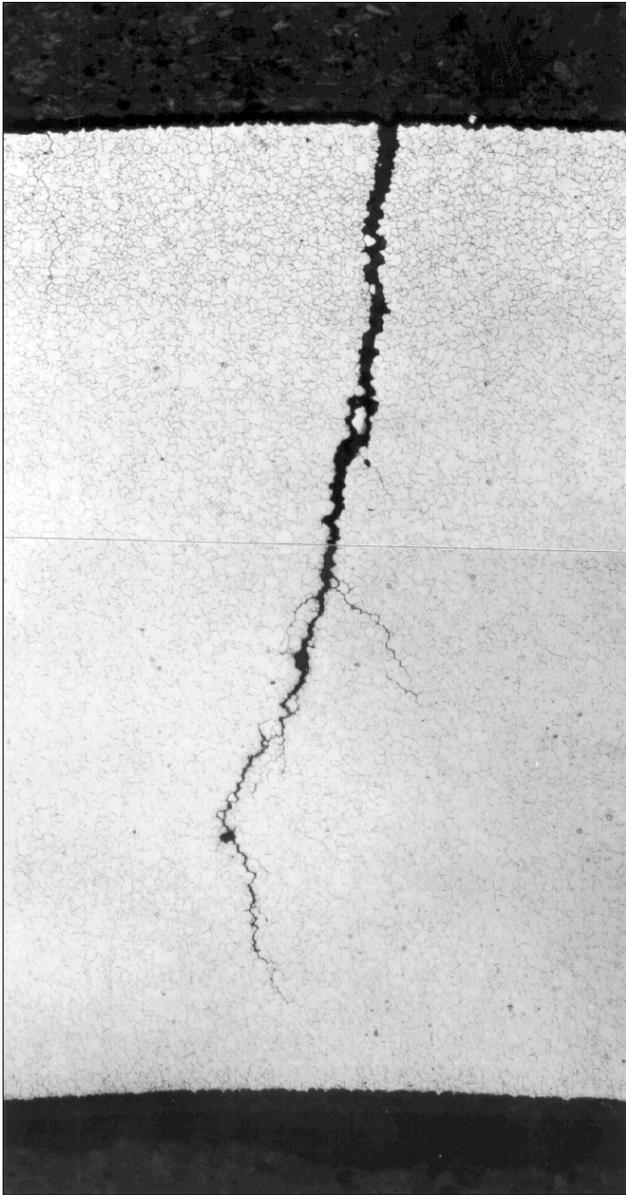
**FIGURE 11.** Alloy 600MA tested in 10% NaOH, plus impurities at  $E_{peak}$  during 250 h (100X).
