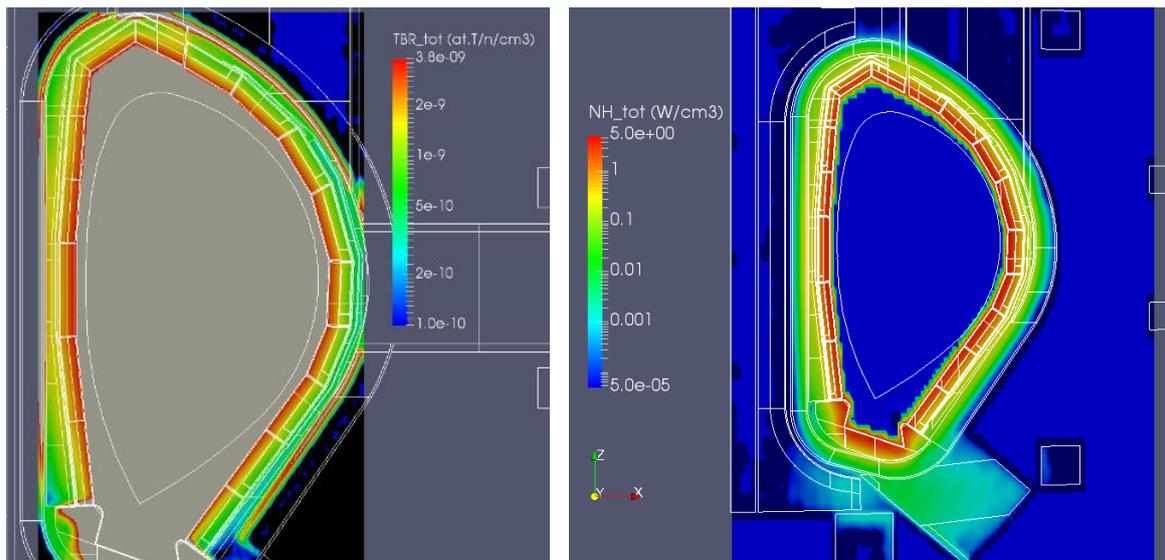
FIG. 2. (left) Radial-poloidal distribution of the tritium generated (at. T/n/cm<sup>3</sup>); (right) radial-poloidal distribution of the nuclear heating (W/cm<sup>3</sup>) in the whole DCLL DEMO.
