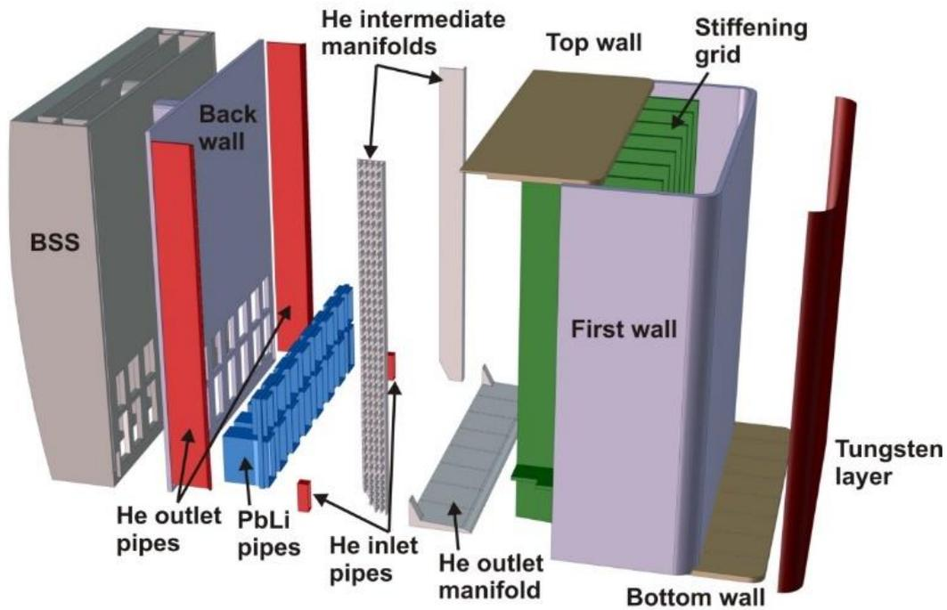
FIG. 1. Distribution of the components in one module of the DCLL breeding blanket.
