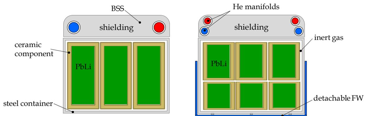
FIG. 16. Cross section of the high temperature breeding blanket showing the different alternatives that could be used for the routing of the different effluents. A detachable FW could be used (right figure), although an integrated FW is preferred (left figure).
