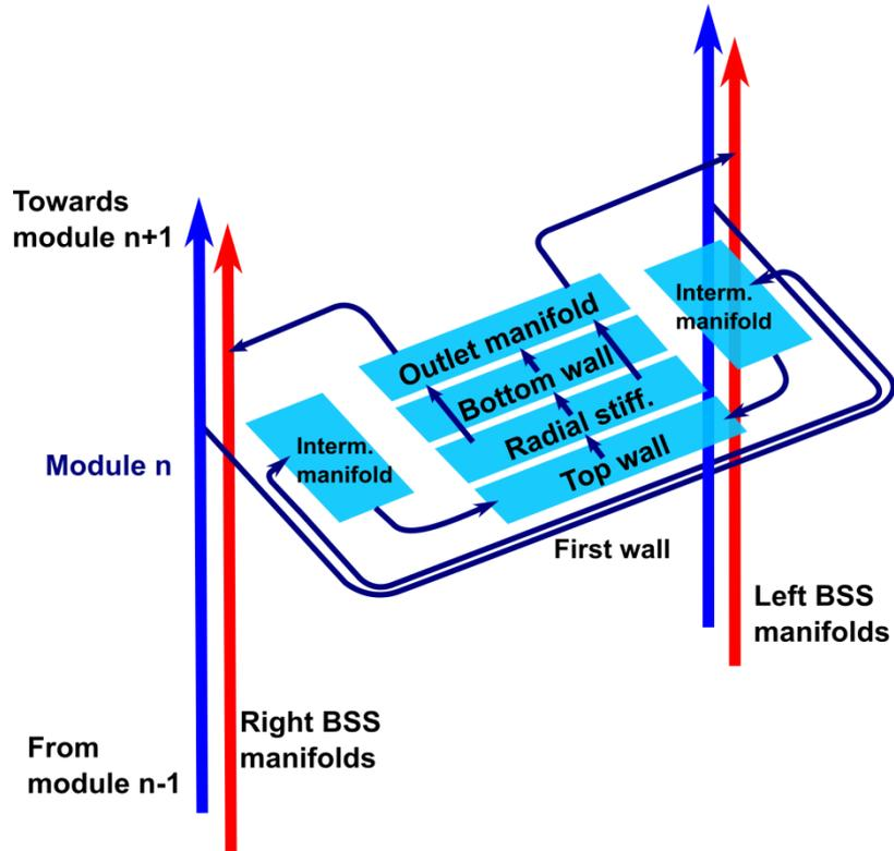
FIG. 4. Scheme of the helium route inside the DCLL module
