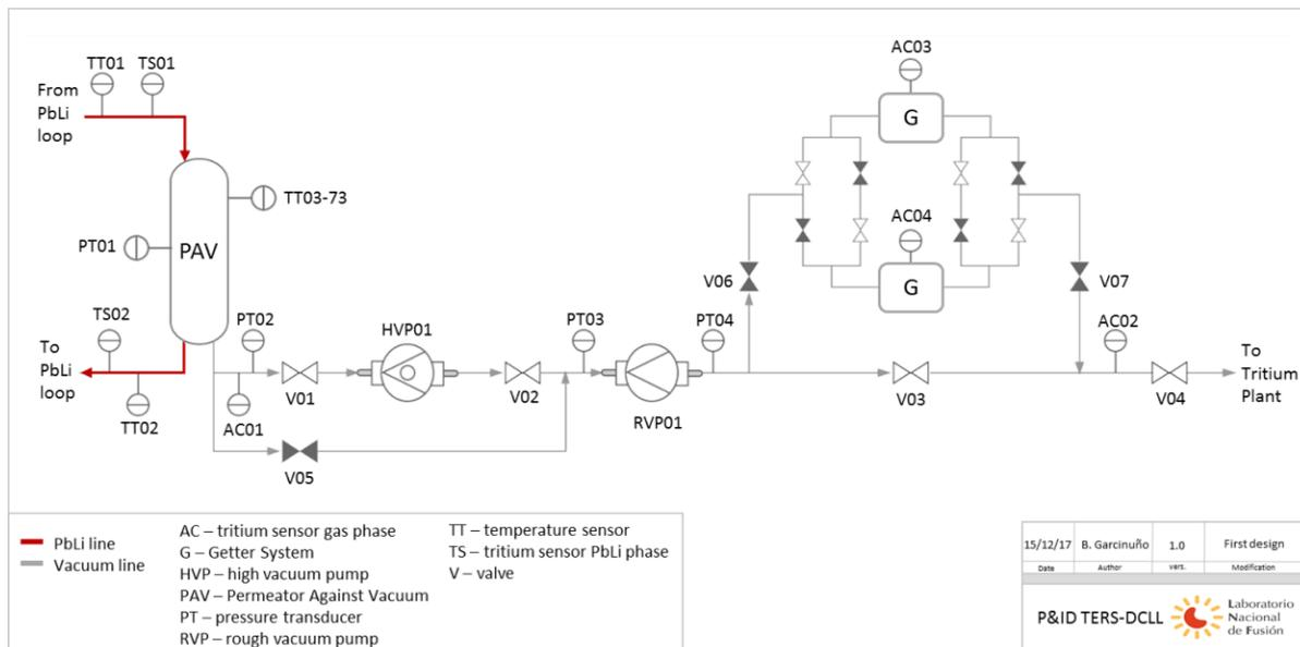
FIG. 9. P&ID of the Tritium Extraction and Removal System for the DCLL DEMO showing its main components: PAV; vacuum system; getter system; temperature sensors; pressure transducers; valves; tritium sensors in gas and PbLi phases.
