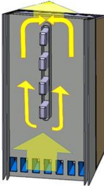
FIG. 14. Sketch of the PbLi circulation around the internal obstacles in one of the BSS manifolds.
