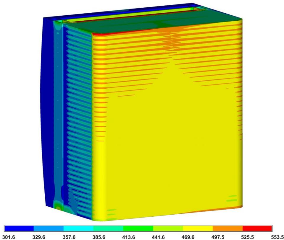
FIG. 3. Temperature map (°C) in the outboard equatorial module (tungsten layer removed).
