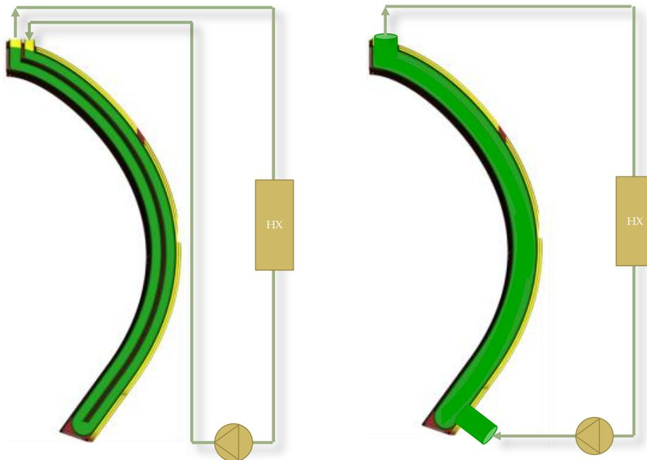
FIG. 15. Schematics showing the possibilities to route the liquid metal in a single-module design.
