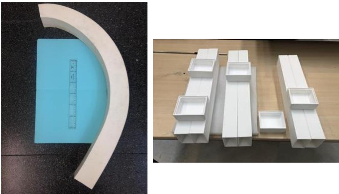
FIG. 6. Left) Final sintered banana-shaped FCI; Right) longitudinal alumina mock-ups produced by casting.
