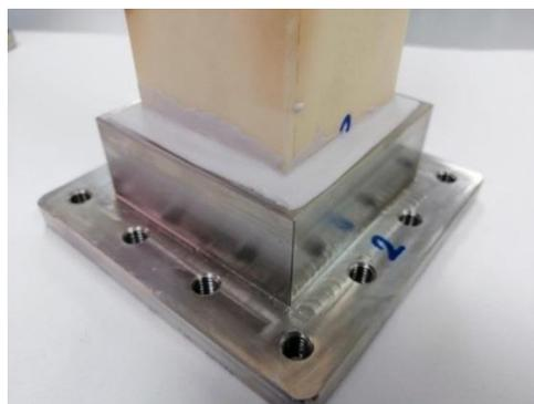
FIG. 7. Prototype assembly of the squared sectioned alumina tube and the steel flange with a white ceramic cement, before being submitted to mechanical stability tests at high temperature.
