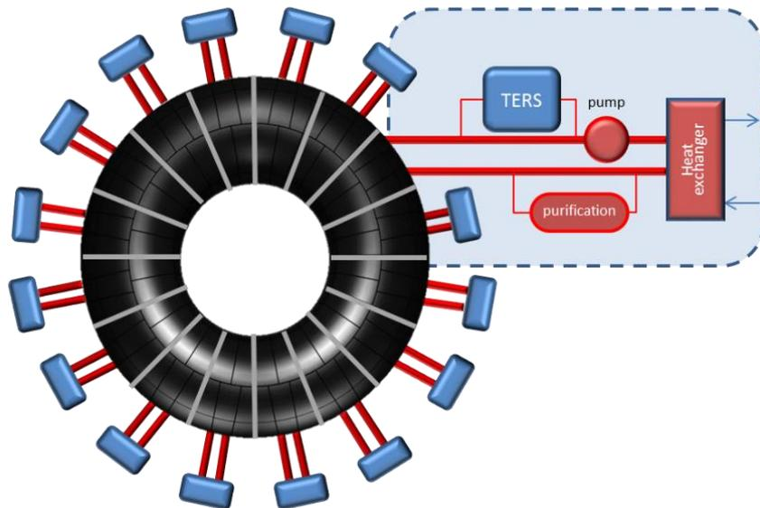
FIG. 8. Toroidal section view of the DCLL DEMO showing the 16 sectors (grey) and the PbLi loops (red). A detail of only one of the PbLi loops, including its main components (TERS - blue, heat exchanger, purification), is shown
