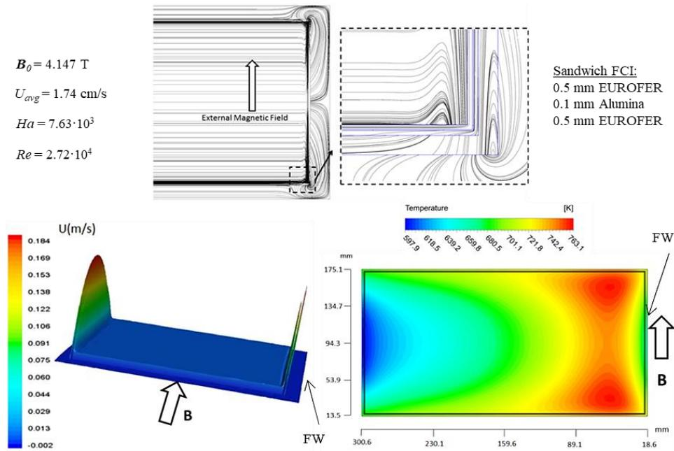
FIG. 5. Main results of the MHD-thermal computations for a channel with a thin sandwich FCI. (top) Electric currents induced in the PbLi channels. (bottom-left) MHD fully developed velocity profile in a frontal PbLi channel. (bottom-right) Temperature distribution in the same channel considering the neutronic volumetric heating.
