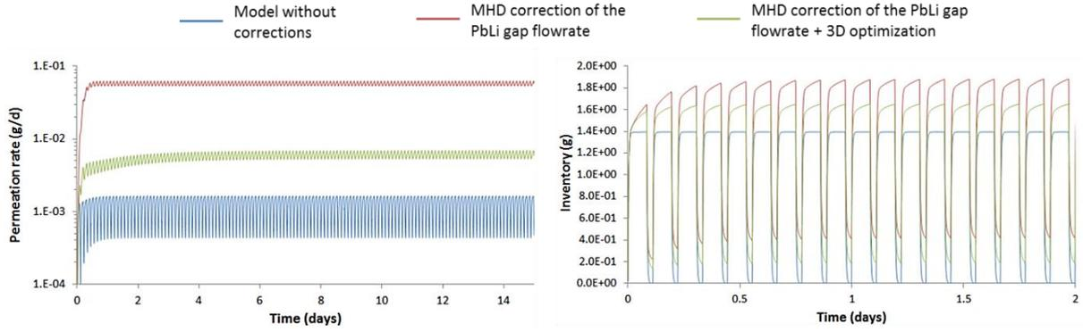
FIG. 13. (left) Total permeation rate from PbLi to He inside the blanket. (right) Total tritium inventory inside the PbLi
