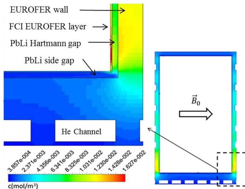
FIG. 12. Tritium concentration contours in the mid-section of the DCLL front channel gap
