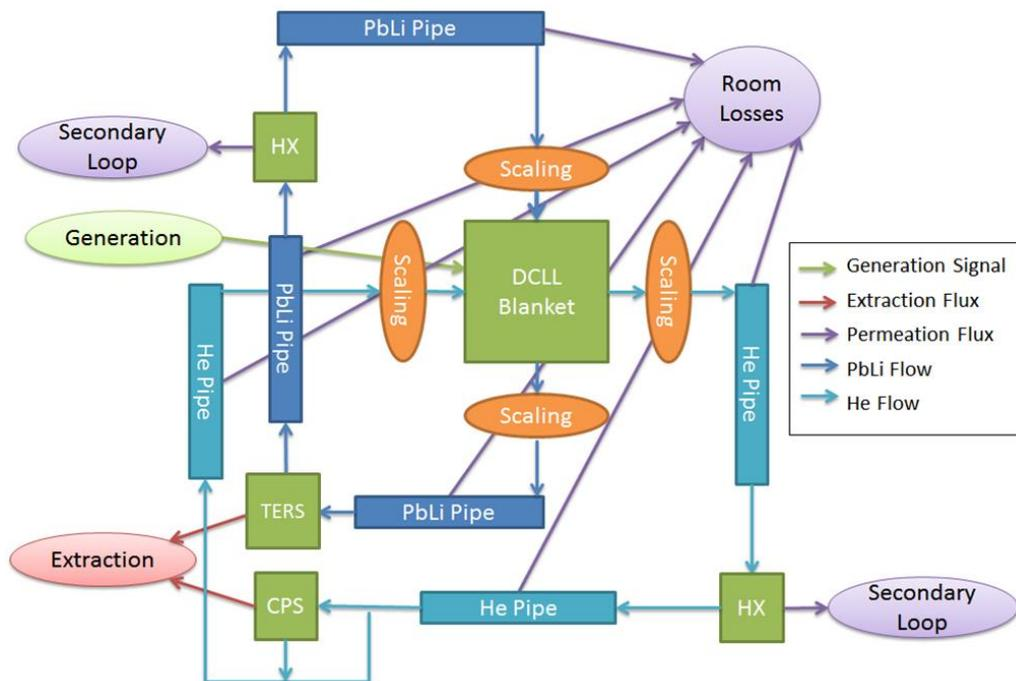
FIG. 11. External Process Flow Diagram of the system level tritium transport model including the blanket and the ancillary systems used to model the blanket and the ancillary systems
