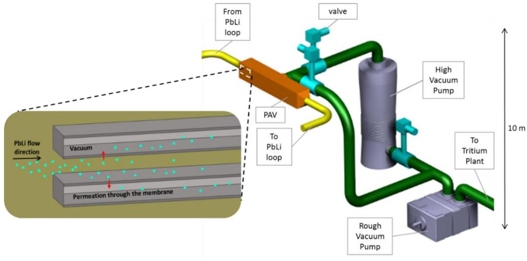
FIG. 10. Schematic view of the working principle of PAV (left) and 3D design of the TERS (right)
