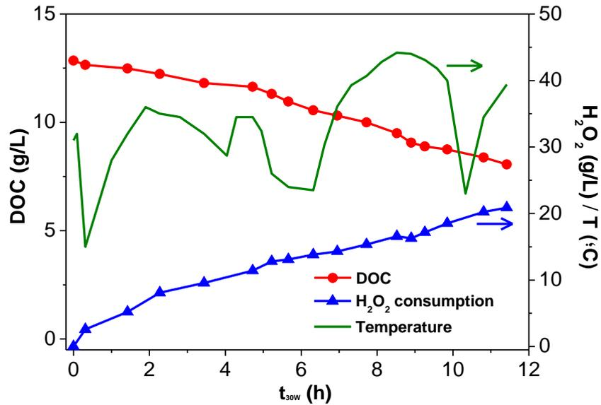
**Figure 2.** Solar photo-Fenton treatment of LL2 with 1 mM of Fe<sup>3+</sup> at CPC pilot plant scale.
