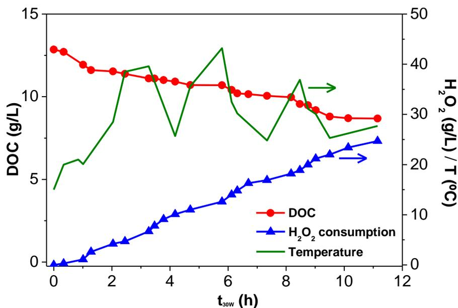
**Figure 3.** Solar photo-Fenton treatment of LL2 with 2 mM of Fe<sup>3+</sup> at CPC pilot plant scale.
