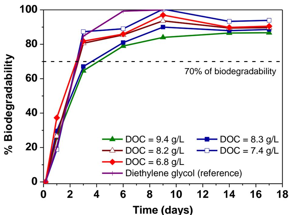
**Figure 5.** Zahn-Wellens test results for samples taken along the solar photo-Fenton treatment of LL2 performed at 1 mM of  $\text{Fe}^{3+}$ .
