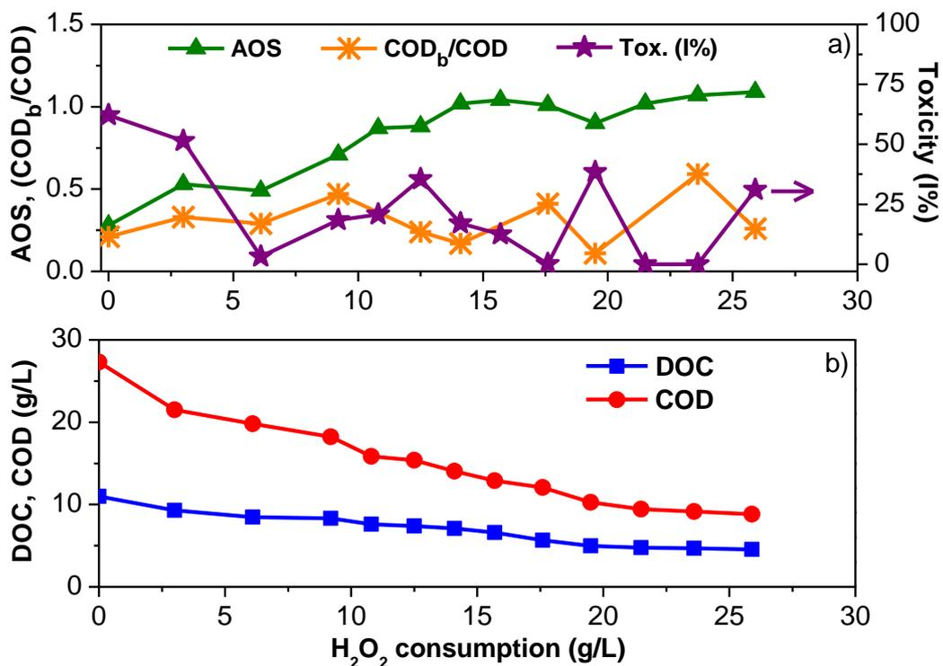
**Figure 1.** Evolution of the main parameters throughout LL1 treatment with solar photo-Fenton process in the solar simulator: **a)** AOS, biodegradability (COD<sub>b</sub>/COD) and toxicity; **b)** COD and DOC.
