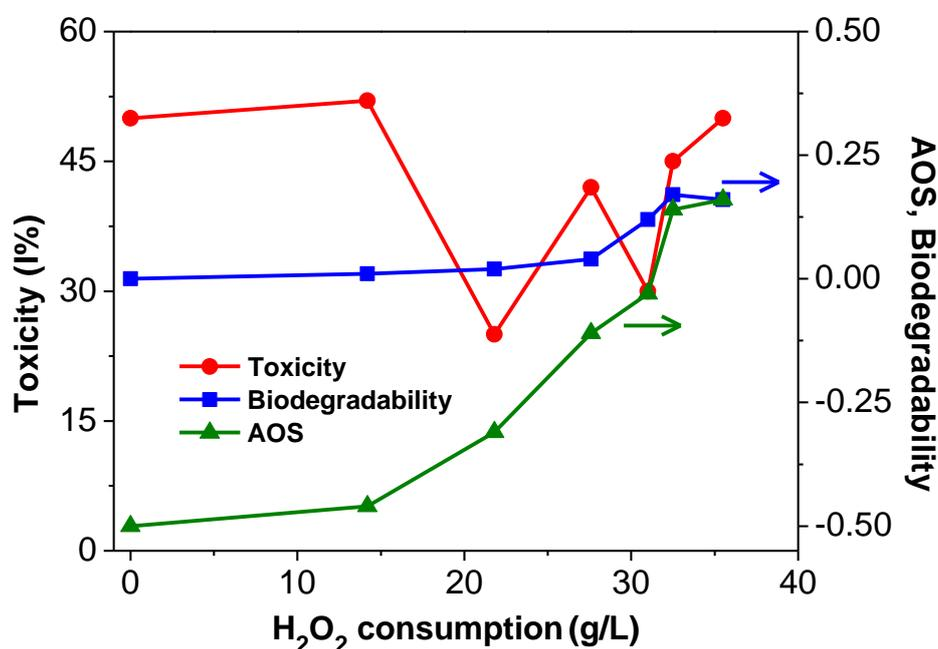
**Figure 4.** AOS, toxicity and short term biodegradability assessment during solar photo-Fenton treatment of LL2 performed at 1 mM of  $Fe^{3+}$ .
