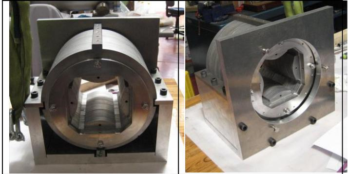
Fig.2. Two different views of the iron yoke stacking tool.
