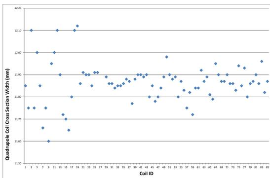
Fig.1. Quadrupole coils cross section width data.
