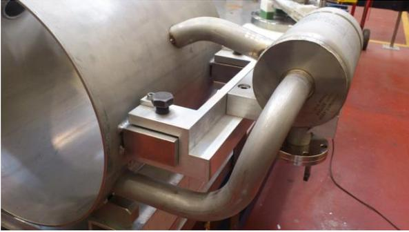
Fig.3. Custom tool for positioning during welding.
