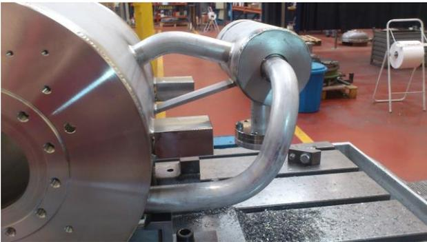
Fig.4. Detail of the bended tube.
