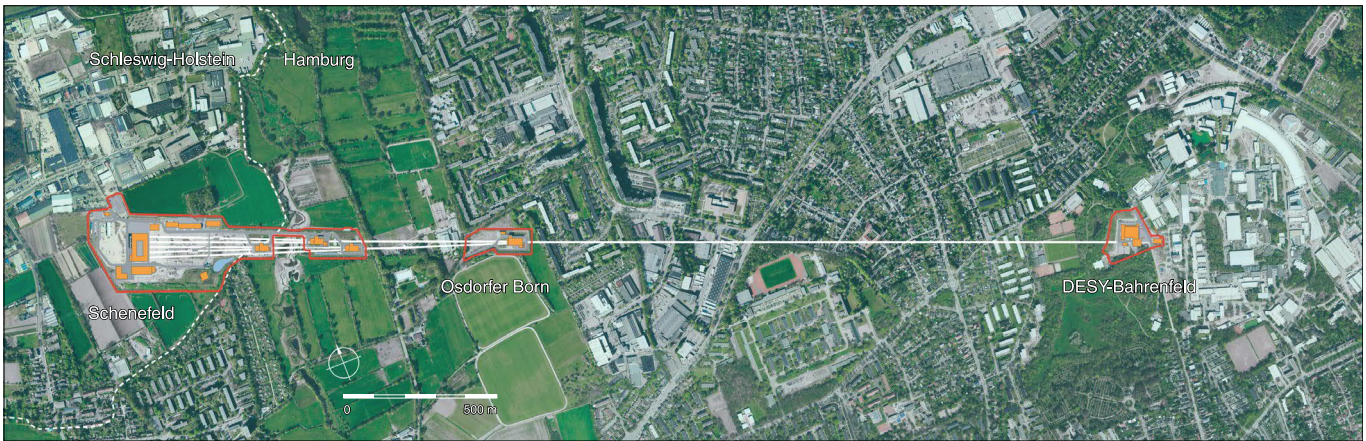
Fig. 1 | Bird's-eye view of the facility showing the location of the tunnel buildings in the urban area of the city of Hamburg. The injector is on the right on the DESY campus, while the experiment hall and headquarters of the European XFEL are on the left in the federal state of Schleswig-Holstein. Note the fan of five photon beamlines entering the experiment hall. Credit: European XFEL / Luftaufnahmen: FHH, Landesbetrieb Geoinf. und Vermessung
