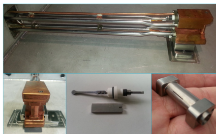
Fig. 2. Pictures of the ion source showing a lateral view with the water cooling pipes and the gas supply pipes (top), a frontal view of the main body of the source and the anode (bottom left), a cathode with electrical insulator (bottom center) and the chimney (bottom right).
