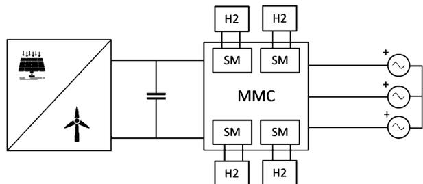
Fig. 1. Proposed green hydrogen generation system
