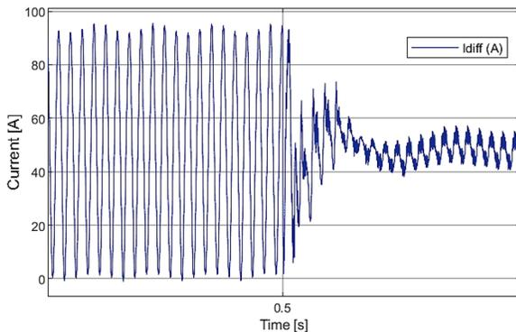
Fig. 6. Simulation of Circulating Current Control
