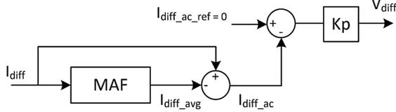
Fig. 5. Circulating current control
