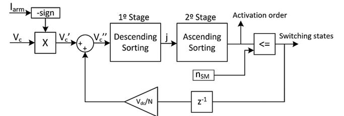
Fig. 7. Voltage Balancing Algorithm
