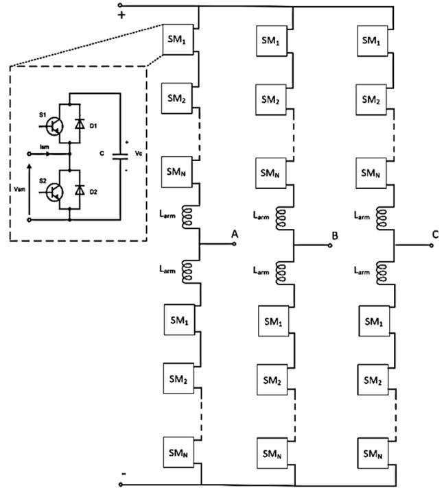
Fig. 3. Three-phase MMC converter
