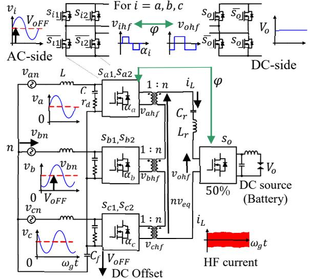
Fig. 3. Proposed QABSR 3P AC-DC converter.
