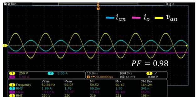
Fig. 9: Grid and DC output currents for B2G.
