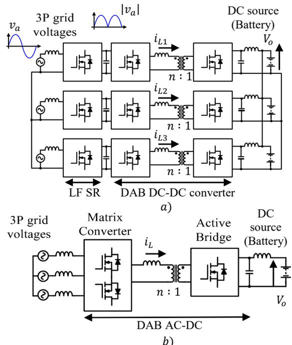
Fig. 1. SS 3P AC-DC converters based on the DAB converter a) Three independent 1P DAB AC-DC converters b) 3P AC-DC DAB converter
