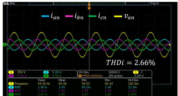
Fig. 9: Grid and DC output currents for B2G.
