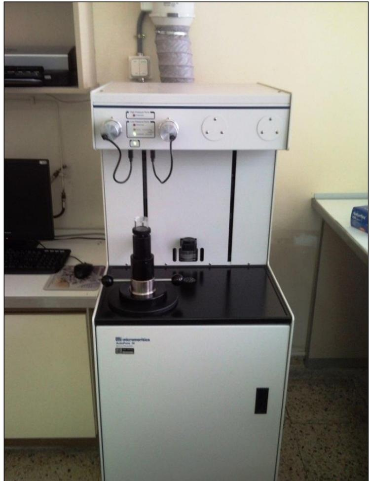
Fig. 3 Hg injection porosimeter AutoPore IV-9500 – Micromeritics. Petrophysics Laboratory (CIEMAT).
