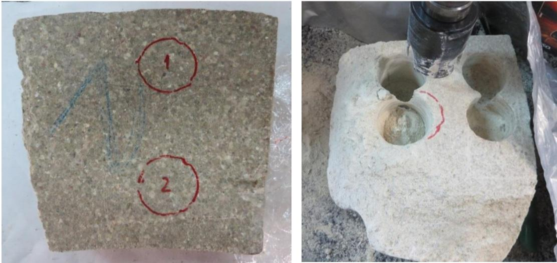
Fig. 8 Location of sampling position in the blocks for the petrophysical, water content and dry density determinations,
