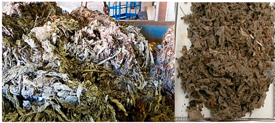
Fig. 1. Cellulosic rejections collected at the wastewater treatment plant “EDAR del Besòs” in Barcelona (left) and the same material upon their arrival at CIEMAT’s laboratories (right).
