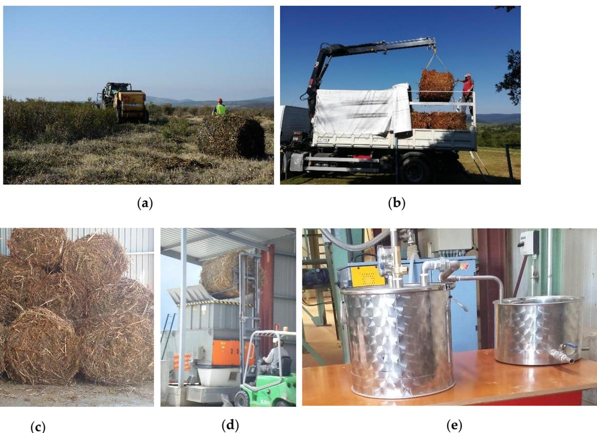
**Figure 2.** Processes carried out during the pretreatment of the plant material: (a) mechanised harvesting of *Cistus ladanifer*, (b) transport of the bales, (c) indoor storage, (d) crushing of the bales and (e) distillation of the milled biomass.
