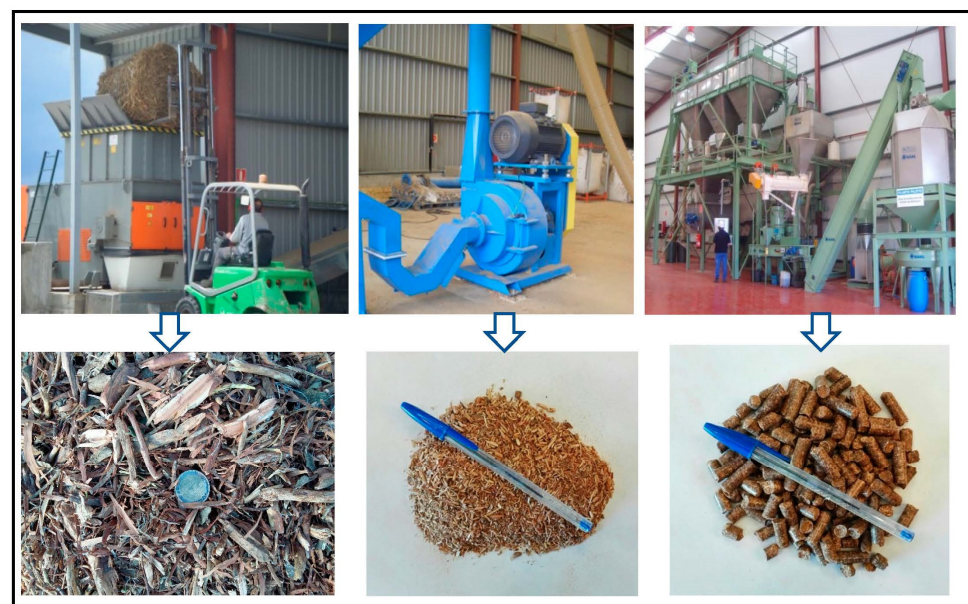
Figure A3. Pre-shredder (90 kW) and 30 mm milled rockrose ( left ); Post-grinder (75 kW) and 4 mm milled rockrose ( center ); Pelletisation pilot plant (30 kW) and Ø 8 mm rockrose pellets ( right ). Installations located at CEDER-CIEMAT (Soria).
