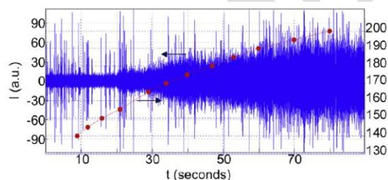
Figure 8 Signal from HP8103 at 108 m<sup>3</sup>/h (band-pass filter 12–13 kHz) and temperature measured at 1 mm from the hot finger tip. As the circuit during the experiments was not completely degassed, air bubbles are seen as short spikes.
