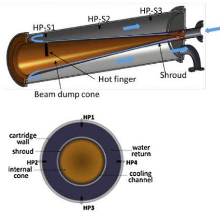
Figure 1 Beam dump cartridge longitudinal and transverse sections showing the positions where the hydrophones will be installed and the hot finger position in the experiments.
