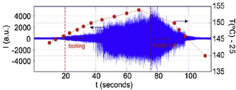
Figure 6 Signal from HP8103 at 25 m<sup>3</sup>/h high pass filtered (500 Hz) and temperatura measured at 1 mm from the hot finger tip.
