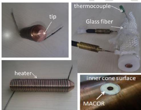
Figure 3 Hot finger. The lower right picture shows it mounted at the cone and viewed from the water side.
