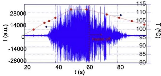
Figure 4 Raw signal from HP8103 for stagnant water conditions and temperatura measured at 1 mm from the hot finger tip.
