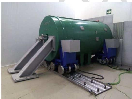
Figure 29 Assembly test of the beam dump shielding.
