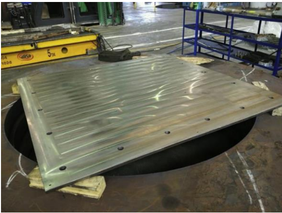
Figure 26 Central base plate after machining.
