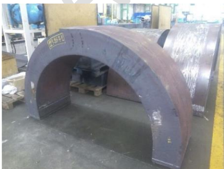
Figure 21 Iron half ring after bending.
