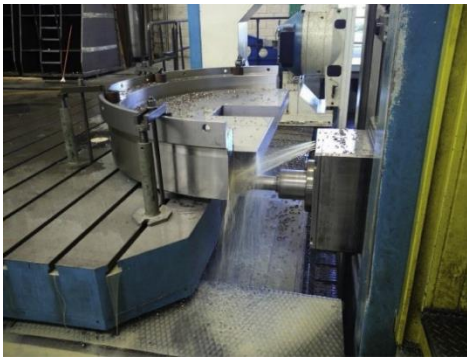
Figure 22 Iron half ring in the milling machine.
