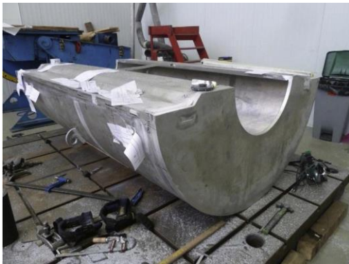
Figure 23 Aluminum tank during the welding stage.
