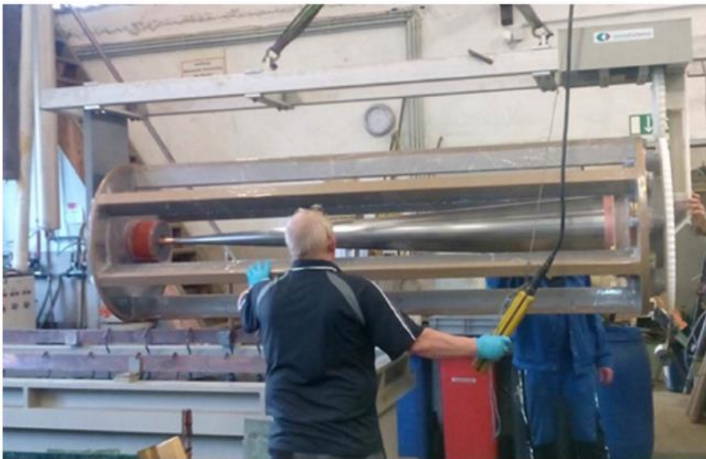
Figure 7 Assembly for electroforming of the cone body. Scheme and picture of its introduction in the electrolytic bath.
