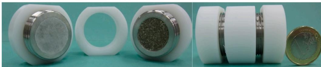
Fig. 1. Picture of the diffusion cell. Left: open cell; Right: assembled cell.
