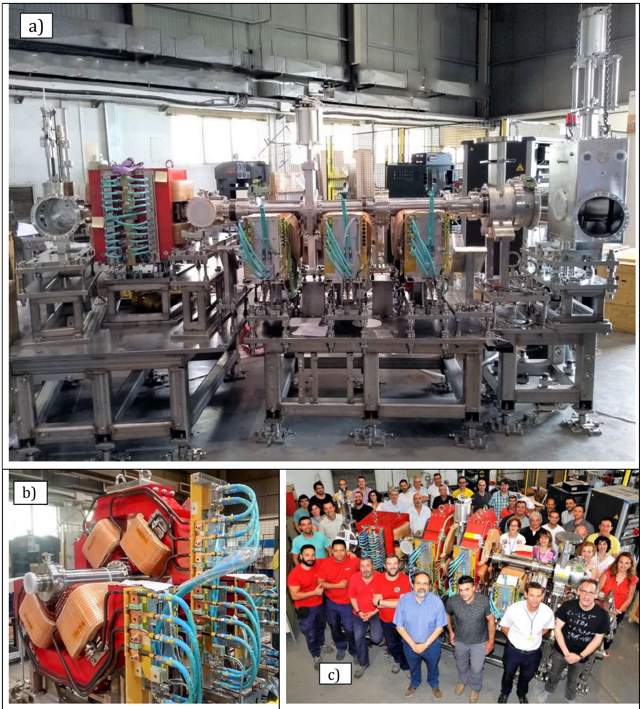
Figure 29: a) The last three subassemblies of the HEBT line partially mounted at CIEMAT premises for assembly tests. The upper halves of the second triplet magnets have been removed for working in the beam tube. b) The first triplet subassembly of the HEBT line with the tube the magnets partially installed. c) CIEMAT team contributing to the design and manufacturing of the HEBT line.
