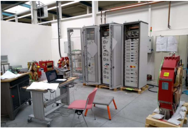
Figure 26: Magnet power supplies during tests at the factory with the real loads
