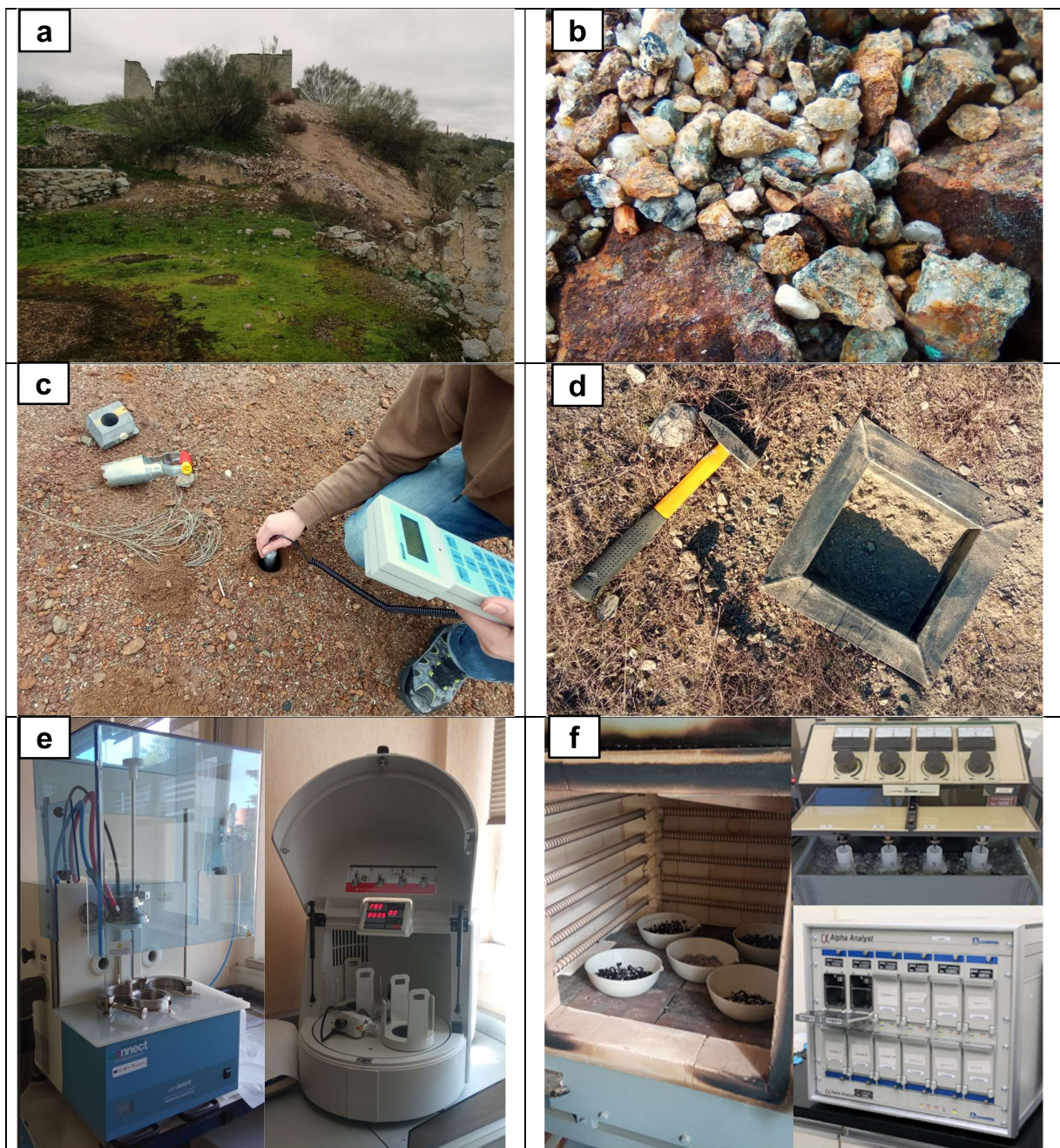
Figure 2. Various stages of the soil and plant sampling and preparation process: (a) the waste rock dump of the “Antigua Pilar” copper mine, (b) a detailed view of the minerals present in the study area, (c) in-situ measurements taken prior to sample collection, (d) soil sampling using a 20 cm × 20 cm × 5 cm depth grid, (e) a microwave oven (Milestone, ultraWAVE, Italy) and an ball mill (FRITSCH, Pulverisette 5, Germany), and (f) amuffle furnace (HOBERSAL, 2003741, Spain) and alpha spectrometry measurement equipment (Mirion Canberra, Alpha Analyst, Bretonneux, France).
