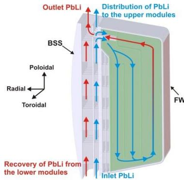
Fig. 2. PbLi routing in the OB equatorial module.
