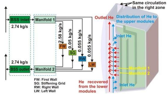
Fig. 3. He cooling scheme in the OB equatorial module.
