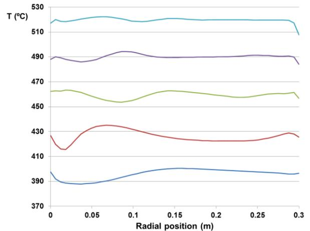
Fig. 8. Temperature profiles along the radial length of the PbLi channel at different poloidal positions ( $t=153$  s). Central vertical plane ( $r=0$  indicates the position of the first wall).
