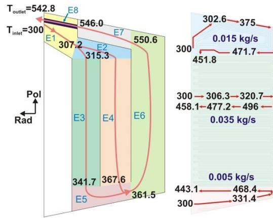
Fig. 5. Evolution of PbLi temperature (°C) along the circuit (left). He temperature (°C) in different locations of a side wall (right).
