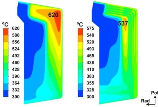
Fig. 6. Temperature map of a radial stiffening plate without He channels (left). Temperature map for 4 channels, 20 m/s and 30 mm pitch (right).
