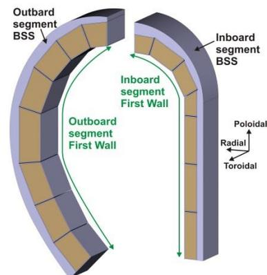
Fig. 1. Shape of the outboard and inboard MMS.
