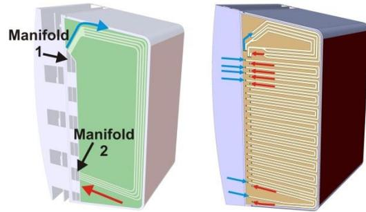
Fig. 4. He cooling channels in the radial stiffening plates (left) and side walls (right).
