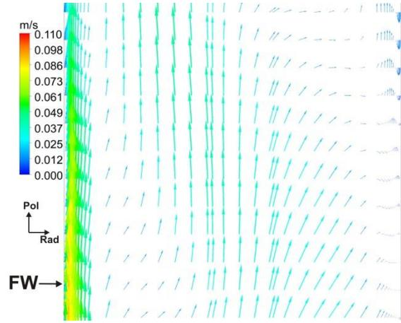
Fig. 7. Velocity vectors in a central vertical plane of the poloidal PbLi channel ( $t=153$  s). Detailed view of the equatorial region.
