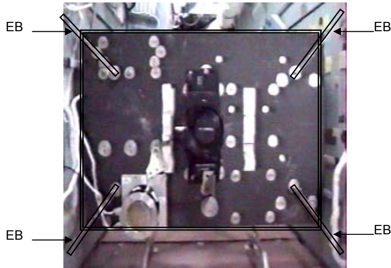
Fig. 1. The facility ALICE-2 is attached to the walls of the “Priroda” module of the Mir station by elastic belts (schematized by EB) and excited at the resonance frequency.
