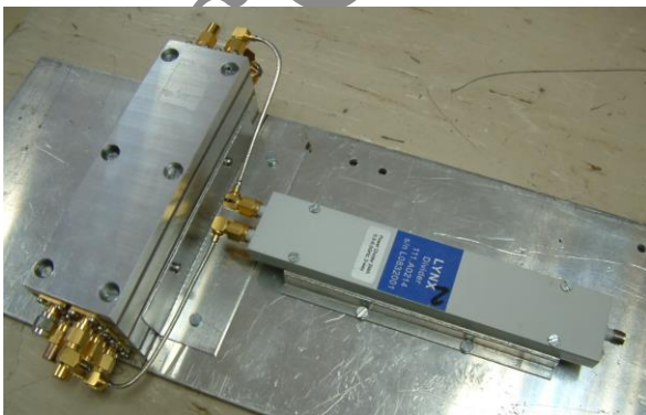
Fig. 7 Six-port network physical realization.
