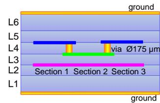
Figure 3. Cross section of the 8.34-dB coupler
