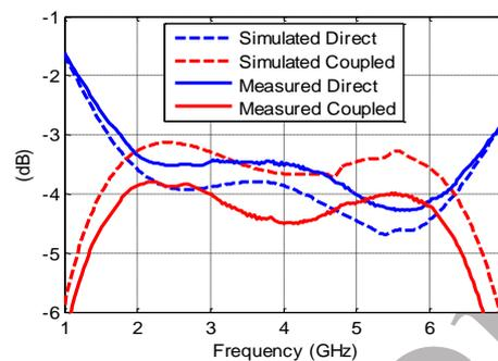
Figure 12. Insertion losses of the LTCC 3-dB tandem coupler
