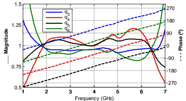
Figure 9. Simulated  $q_i$ -points of the LTCC six-port network
