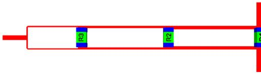
Figure 5. Layout of the Wilkinson power divider
