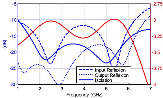
Figure 6. Simulated frequency response of the Wilkinson power divider
