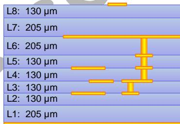
Figure 2. LTCC layer structure
