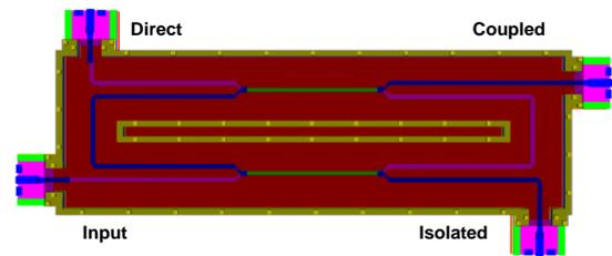
Figure 4. Top view of the LTCC 3-dB tandem coupler
