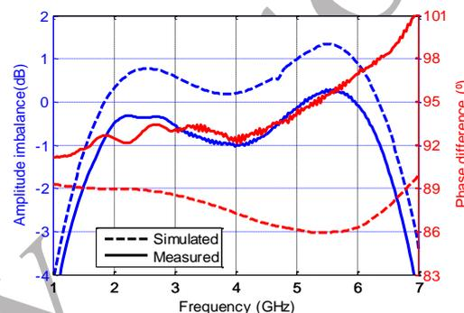
Figure 13. Amplitude and phase imbalances of the LTCC tandem coupler
