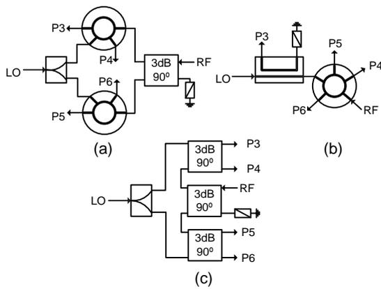
Figure 1. Examples of six-port network topologies
