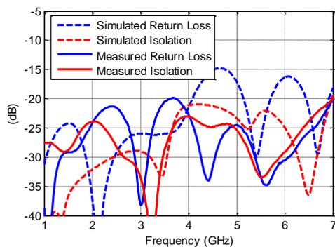
Figure 11. Input return loss and isolation of the LTCC 3-dB tandem coupler
