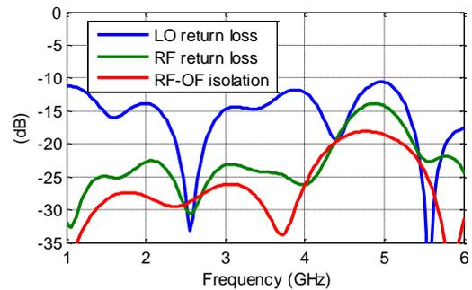
Figure 8. Simulated return losses and isolation of the LTCC six-port network
