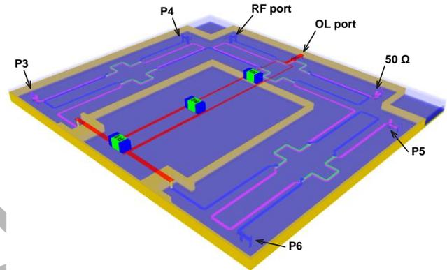
Figure 7. 3D view of the LTCC six-port network
