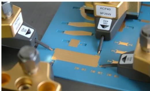
Figure 10. Fabricated LTCC 3-dB tandem coupler
