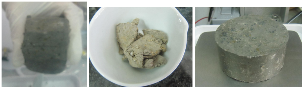
Fig. 6: Appearance of the sample QT-C5 from m.32-33: a) initial sample, b) initial sample after drying at 110 °C for water content determination prior to the squeezing test, and c) sample after squeezing.
