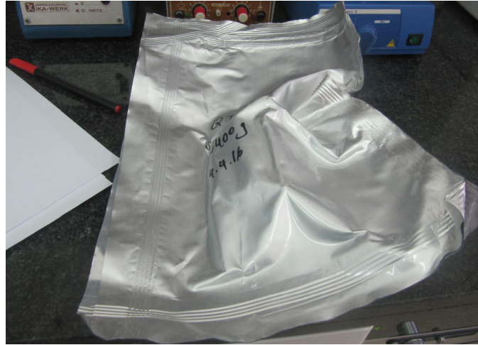
Fig. 1: Drillcore samples preserved at vacuum in Al-foil bags.
