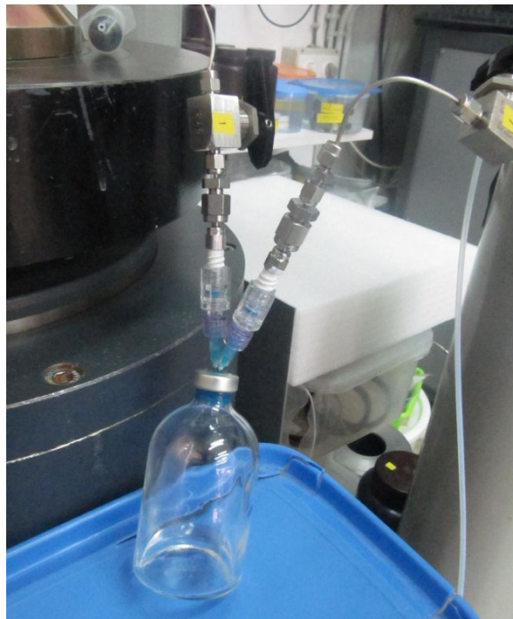
Fig. 3: Vacuum vials for collecting pore water preserving the anoxic conditions.
