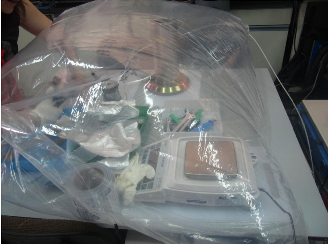
Fig. 4: Anoxic glove bag flushed with Ar for preparing the sample and the cell prior to the squeezing tests.
