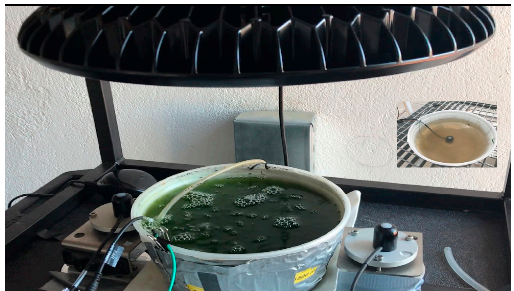
Figure 1. Experimental start-up of microalgae cultivation in domestic wastewater.
