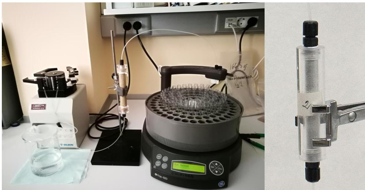
Figure 5. Typical set-up for a column experiment with crushed materials and a detail of the column filled by the adsorbent (right).
