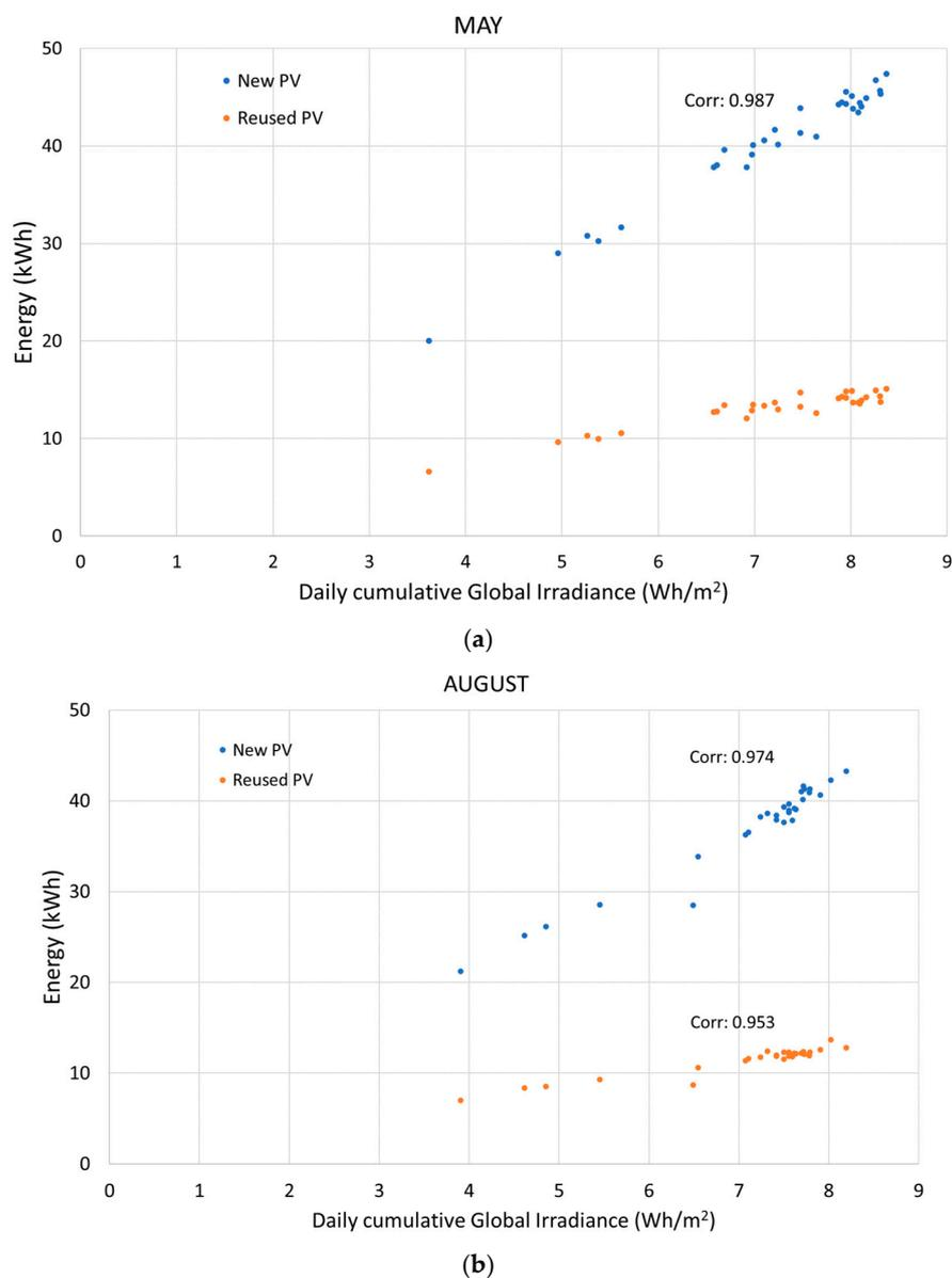
**Figure 9.** Relationship between daily cumulative global irradiance and energy output for new and reused PV panels for (a) May and (b) August.
