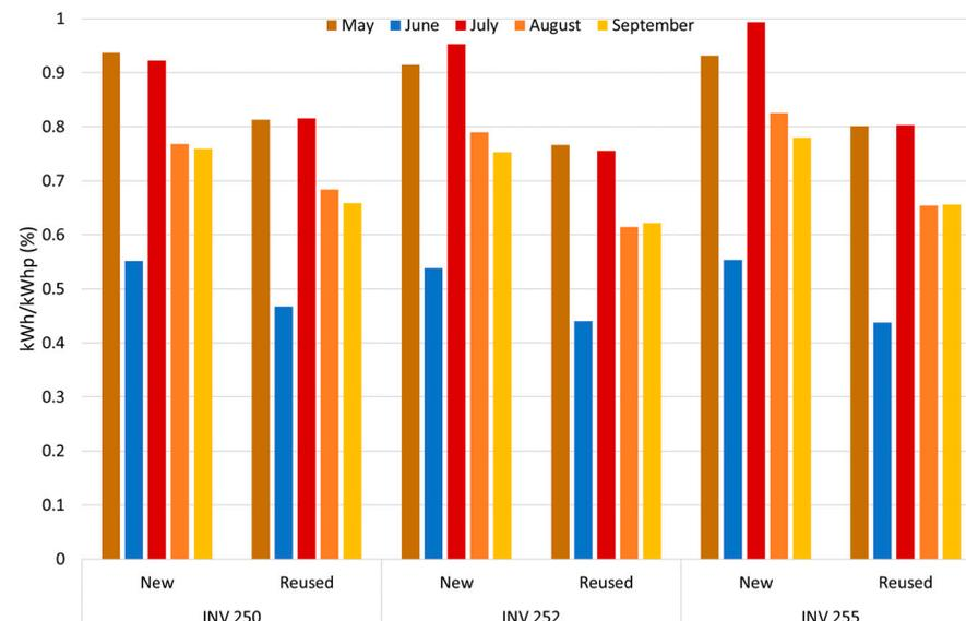
**Figure 8.** Monthly energy production comparison in kWh/kWhp (%) of new and reused PV panels across three inverters.
