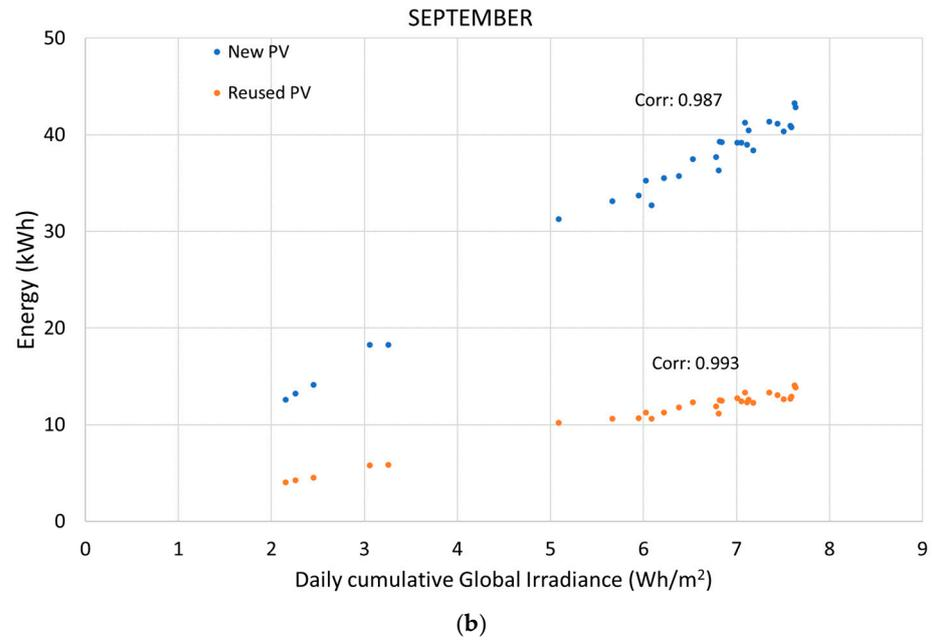
**Figure A1.** Relationship between daily cumulative global irradiance and energy output for new and reused PV panels for (a) July and (b) September.
