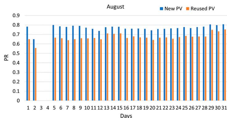
**Figure 10.** Daily performance ratio (PR) of new and reused PV modules in August.
