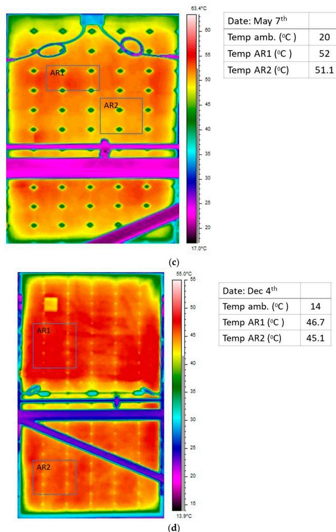
**Figure A3.** IR thermographic images of new PV panels and reused PV panels captured through different months. All temperatures marked in the figures are medium temperatures. (a) New PV panel in 12 March, (b) reused PV panel in 12 March, (c) reused PV panel in 7 May, and (d) new PV panel in 4 December.
