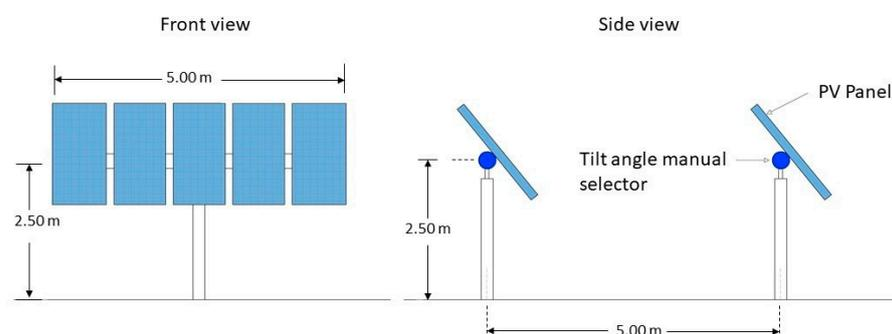
**Figure 1.** Schematic representation of the PV system structure with an adjustable tilt angle: front and side views.
