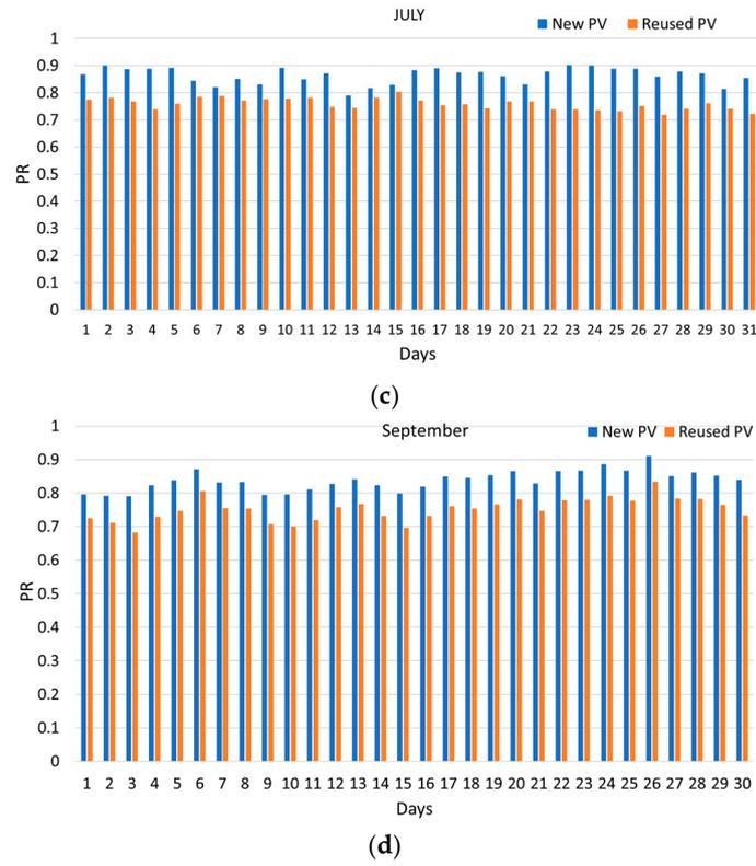
Figure A2. Daily performance ratio (PR) of new and reused PV modules in (a) May, (b) June, (c) July, and (d) September.
